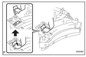
(f) Pull out the connector while pinching the latch with fingers and disconnect the steering pad switch cable from the steering pad switch LH.
