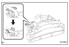
(c) Install the tab of the steering pad switch cable onto the steering pad switch LH as shown in the illustration.
