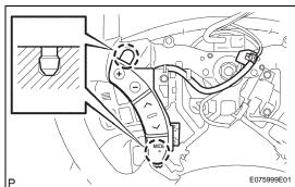
(d) Release the tab of the steering pad switch cable from the steering pad switch LH as shown in the illustration.
