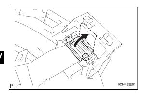
(e) Disengage the 2 claws and open the latch on the top of the connector as shown in the illustration.
