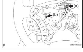
(c) Disengage the 2 pins and remove the steering pad switch LH.
