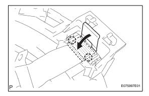
(b) Hold the connector cover down to engage the 2claws as shown in the illustration.
