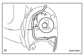
(2) Engage the 4 claws and install the front seat side air bag wire.
