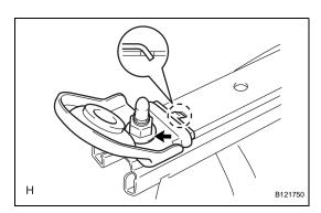
13. INSTALL FRONT SEAT TRACK FRONT BRACKET LH(a) Engage the hook and install the front seat track front bracket with the nut.
