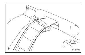
(h) Install the belt of the front center seat outer belt into the front center seat outer belt guide.
