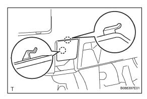
(b) Engage the 2 claws and install the hood lock control lever sub-assembly.
