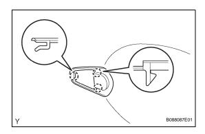
(b) Disengage the 3 claws and remove the front door outside handle front pad.
