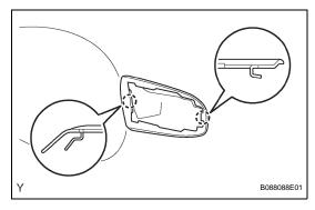
(c) Disengage the 2 claws and remove the front door outside handle rear pad.
