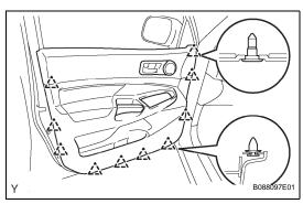
(c) Disengage the 10 clips and remove the front door trim panel assembly LH.
