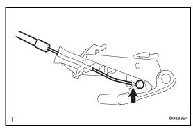
(b) Disconnect the hood lock control cable assembly and remove the hood lock control lever subassembly.
