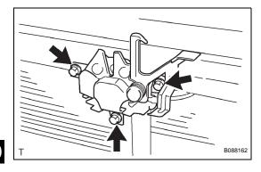
(b) Disconnect the hood lock control cable assembly, then remove the hood lock assembly.
