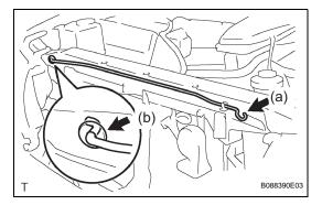
(c) Using a clip remover, disengage the 2 claws and remove the hood stay holder.
