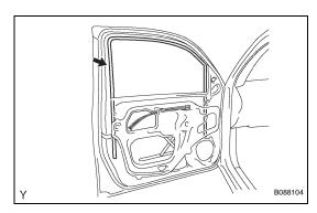
(c) Insert the front door window regulator into the door panel. Use bolt A to hang the front door window regulator on the door panel.
