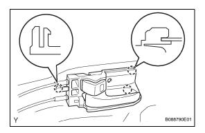
(b) Engage the 3 claws and install the front door inside handle sub-assembly LH onto the door panel.
