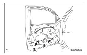
(b) Install the front door glass sub-assembly LH into the front door window regulator sub-assembly LH with the 2 bolts.
