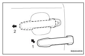
(c) Pushing the front door handle assembly outside LH in the direction of the arrow marks shown in the illustration, install the front door outside handle assembly LH.
