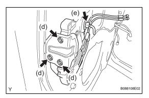
(c) Apply adhesive to the threads of the 3 screws.
