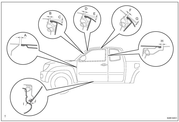
(a) Check that the clearance measurements of areas A to J are within the standard ranges.
