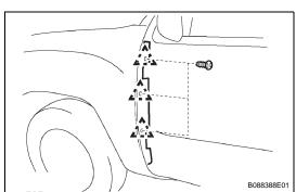
(e) Using SST, adjust the door horizontally and vertically by loosening the body side hinge bolts.SST 09812-00010
