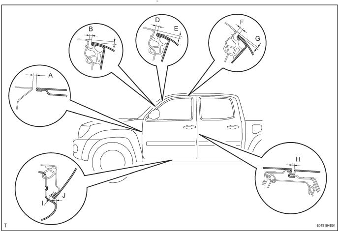
Check that the clearance measurements of areas A to J are within the standard ranges.
