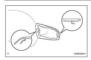
(b) Engage the 2 claws and install the front door outside handle rear pad.
