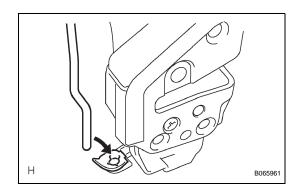
(c) Apply adhesive to the threads of the screws. Adhesive:
