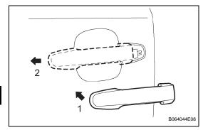
(c) Pushing the front door outside handle assembly LH in the direction of the arrow marks shown in the illustration, install the front door outside handle assembly LH.
