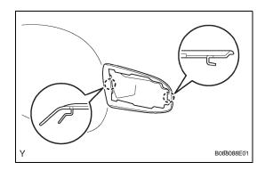
(b) Engage the 2 claws and install the front door outside handle rear pad.
