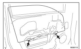
(b) Install the front door glass sub-assembly LH onto the front door window regulator sub-assembly LH with the 2 bolts.
