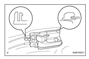
(b) Engage the 3 claws and install the front door inside handle sub-assembly LH onto the door panel.
