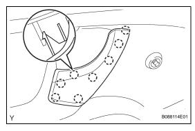
(c) Engage the 8 claws and install the door assist grip cover LH.
