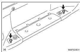
(e) Remove the 2 nuts from the rear bumper bar.
