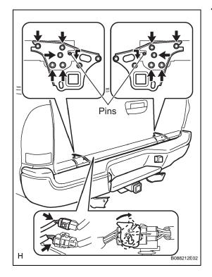
(3) Engage the 3 claws and remove the receiver hitch cap. HINT:
