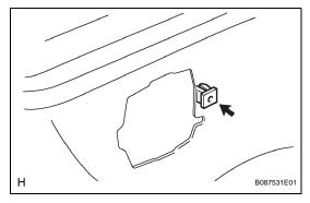
(d) Remove the nut from the rear bumper bar.
