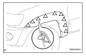
(3) Engage the 9 clips and install the front fender wheel opening moulding.
