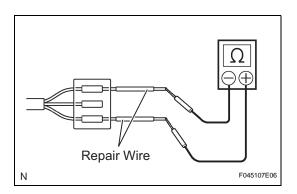
(b) Use a repair wire to check the connector if it is impossible to check continuity from the rear of the connector.
