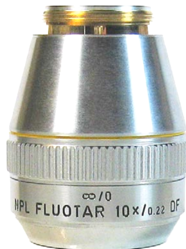
Leitz Wetzlar Germany, 569232, NPL Fluotar 10X/0.22 DF, ∞/0. c1995. This is a normal field of view plan (NPL), fluorite, infinity-corrected objective for dark field (DF) microscopy. 42mm.
