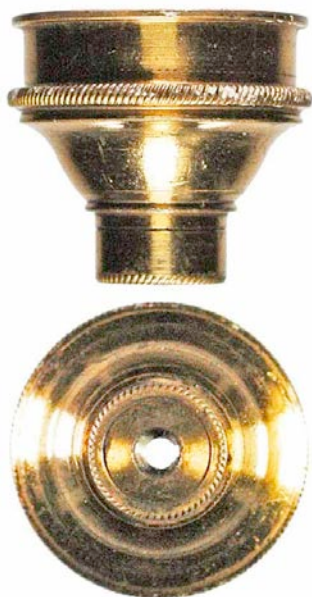
Unmarked. 1760-1790. An objective for a Culpeper-type or Cuff-type microscope. 17 mm w x 15 mm h.
