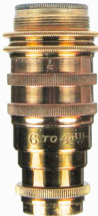
6 TO 4 in, 4 5 6. "R.G. Mason, Clapham, S.W., 6 TO 4 in" on lid. c1890. Continuously variable 6 to 4 inches. Robert George Mason (1849-1912) was a microscope manufacturer and preparer of microscope slides during the last decades of the 19 th century and the early years of the 20 th . 48 to 56 mm.
