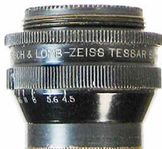
Bausch & Lomb - Zeiss Tessar Series 1c Pat Feb. 24 1903 1305855 48 mm., f-16 11 8 5.6 4.5. Iris diaphragm, RMS threads. This low power, wide field micro-Tessar lens was used as an objective lens for projection setups and microphotographic work with bellows cameras. Used today in digital macrophotography. 22mm.
