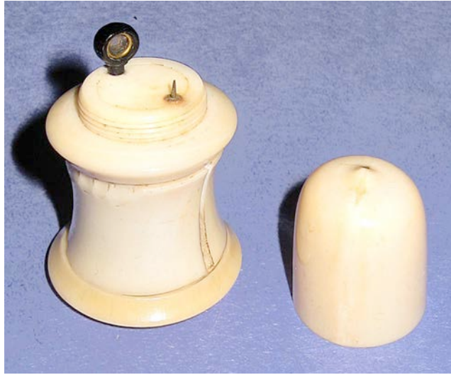
Flea Glass/Acorn Microscope, c1750
