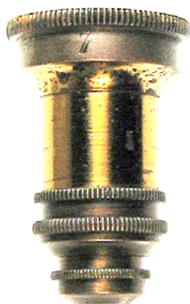
Triplet button objective with 2 screw-on lenses. Marked "7" on objective and canister lid. c1840. Objective has internal female thread i.d. 0.485 in. 29mm.
