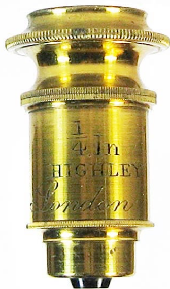
1/4 In, Highley, London. c1855. 5/32 inch internal thread. Samuel Highley manufactured microscopes in the 1850s and 60s. 41mm.
