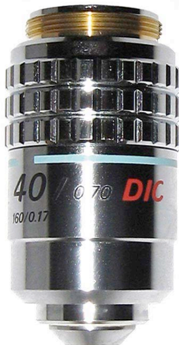
Nikon, Japan, 240774, Plan 40/0.70 DIC, 160/0.17. c1995. Objective for differential interference contrast (DIC) microscopy. 49mm.
