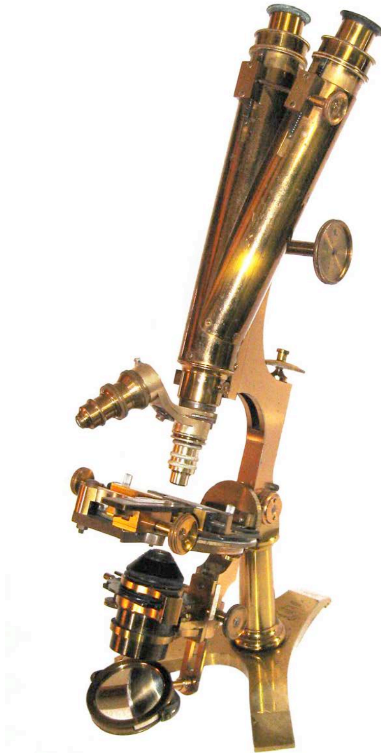
Zentmayer U. S. Army Hospital Binocular Microscope
