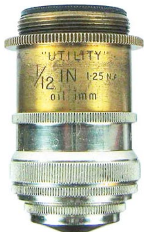
"Utility", 1/12 IN, 1.25 N.A, oil imm, 1.25 .75 .25 N.A. "W. Watson & Sons, Ltd." on lid. c1940. Iris diaphragm for darkfield work. 39 mm.
