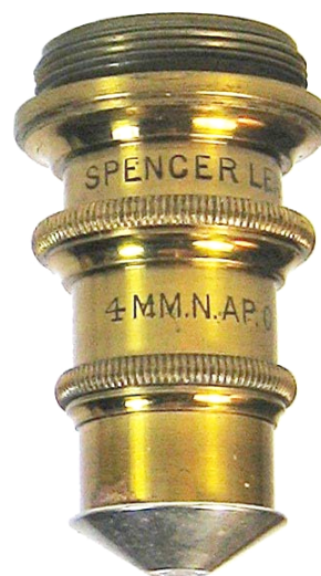
Spencer Lens Co. 50236, 62X, 4 MM.N.AP. 0.75. c1910. The Spencer Lens Company was incorporated in 1895 and was one of two American microscope makers to survive into the 20 th century. 40mm.
