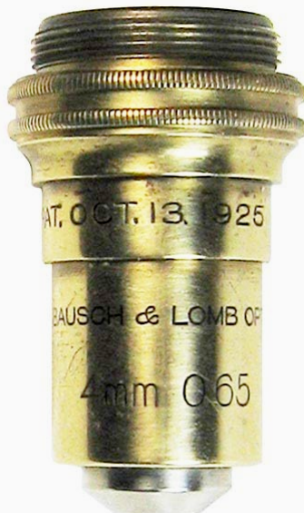
Bausch & Lomb Opt. Co., Rochester N.Y. U.S.A., 43X 4mm 0.65, Pat. Oct. 13 1925. 40mm.
