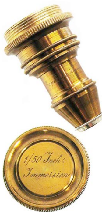
Engelbert & Hensoldt, XIV Immersion. "1/50 Inch Immersion" on canister lid. Correction collar. Louis Engelbert (1814-1887) and Moritz Hensoldt (1821-1903) worked together in Germany from 1852 to 1887. 38mm.
