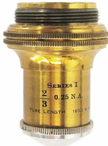
Bausch & Lomb Optical Co. Rochester, N. Y. and New York City, Series I, 2/3 0.25 N. A., Tube Length 160.0 M. M. c1885. 34mm.
