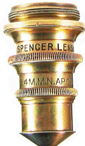
Spencer Lens Co. 73348, 4M.M.N.AP.0.85 Y.U.15 44X. c1915. 37 mm.
