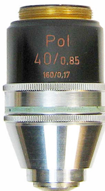
Carl Zeiss, 4403027, Germany, Pol, 40/0.85, 160/0.17. c1995. Spring loaded. An objective for a polarizing microscope. 48mm.
