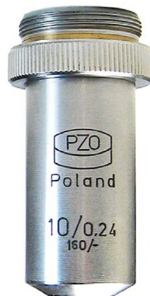
PZO, Poland, 10/0.24, 160/-, 97016. c1980. The precursor of the Polish Optical Industries (PZO) produced its first microscopes in 1926. 46mm.
