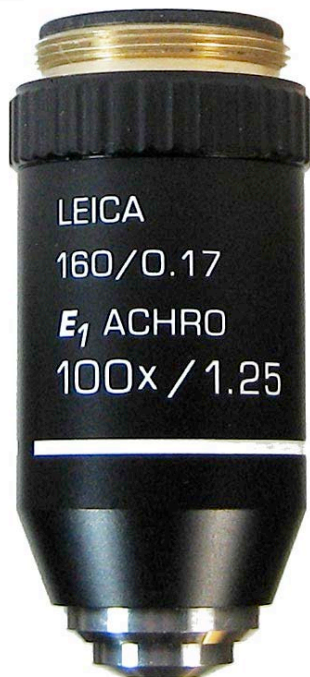
Leica, 160/0.17, E 1 Achro, 100X/1.25, 13394015. c2010. Leica Microsystems emerged in 1997 through mergers and acquisitions from five brand names: Wild, Leitz, Reichert, Jung, and Cambridge Instruments. 50mm.
