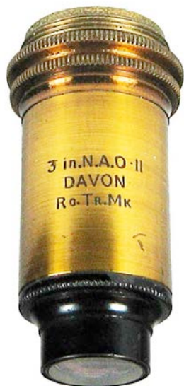
3 in. N.A. 0.11, DAVON, R.G. TR. MK. c1910. The F. Davidson & Co. in London patented the "Davon micro-telescope" in the early 1900s. 45 mm.
