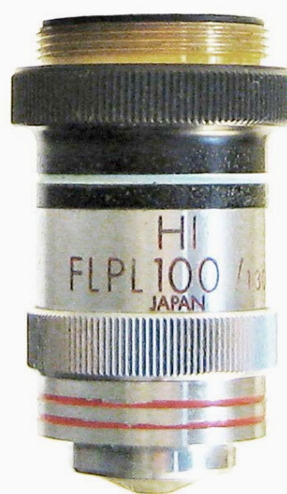
Olympus Tokyo, HI, FLPL 100 / 1.30, Japan, 400243. Internal iris diaphragm. C1990. A 100X, phase contrast, fluorite objective with an iris diaphragm to increase contrast and change numerical aperture. Olympus, a Japanese company, began marketing scientific products in the United States in 1968 and is known as The Olympus Corporation of the Americas. 42mm.
