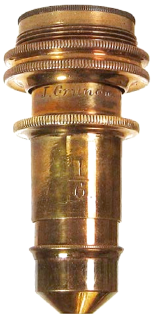
J. Grunow. N. Y., 1/6. Correction collar. c1880. The J. & W. Grunow Co, begun by Julius and William Grunow, was the second microscope manufacturing firm in the U. S. They operated in New Haven around 1854 and moved to New York in 1864 and in 1874 the firm became J. Grunow. 48mm.
