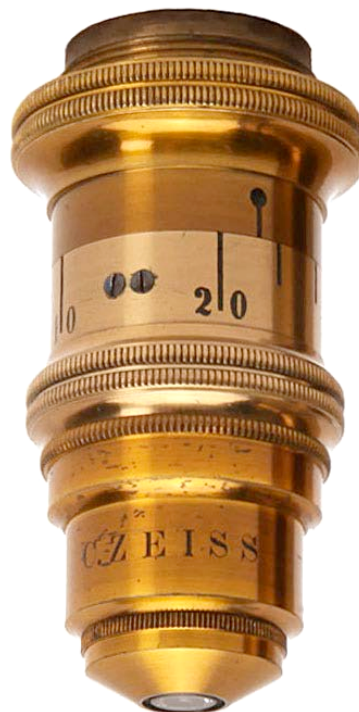
C. Zeiss CC. Correction collar. c1890. Carl Zeiss (1816-1888) opened a mechanical workshop in Jena Germany in 1846 and offered his first compound microscope in 1857. With Ernst Abbe (1840-1905) and Otto Schott (1851-1935), he produced the first apochromatic objectives in 1886. 53mm.
