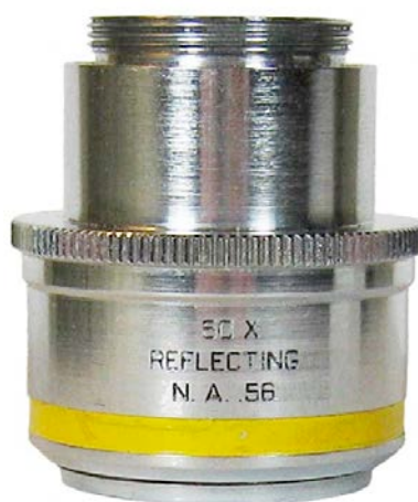
AO Spencer, Made in USA, B31841, 50X, Reflecting, N. A. .56. c1958. A reflecting objective by the American Optical Company. 35mm.
