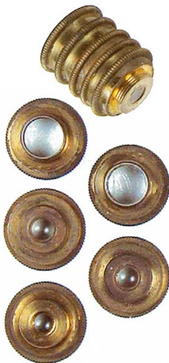
Unmarked five button objective with a 1/4 in female thread. c1820. This type of objective was used on some Cary-Gould and drum microscopes. 13 mm.
