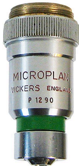
Microplan, Vickers England, P 12 90, 40/0.65, Met. c1990. Spring loaded. This plan objective was designed for a metallurgical microscope using incident light. In 1963, following the acquisition of the C. Baker Ltd. microscope factory, the company of Vickers Instruments was formed in York. England. 47mm.
