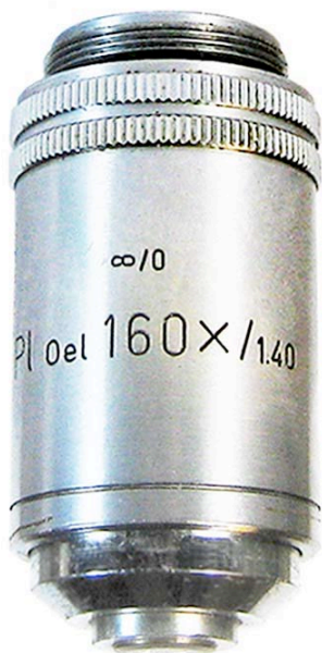
Leitz Wetzlar, C 11256, Germany, ∞/0, Pl Oel, 160X/1.40. c1995. Spring loaded. This oil immersion, infinity-corrected, plan objective represents the maximum practical magnification (160X) and numerical aperture (1.40) achievable for an objective. 50mm.
