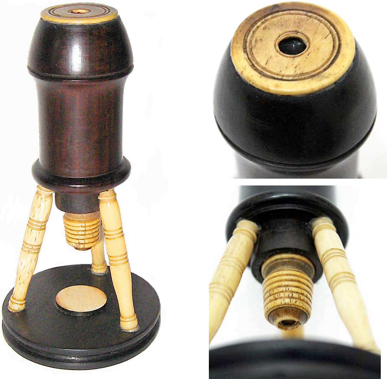
Compound Tripod Microscope, Second Half Seventeenth Century
