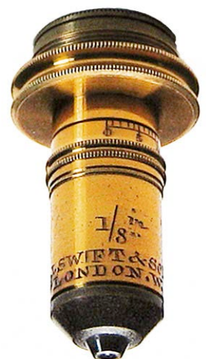
J. Swift & Son, London. W., 1/8 in. Correction collar. c1890. James Swift founded his firm in 1857 in London and was joined by his son in 1884. 44mm.
