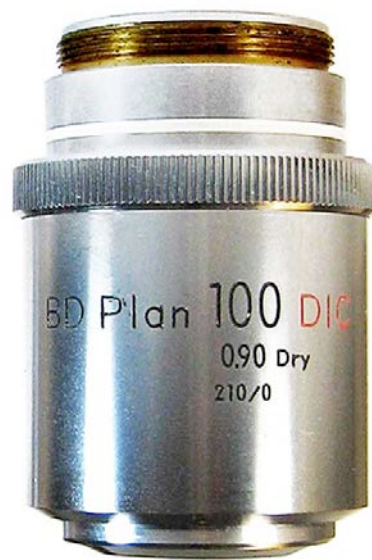
Nikon 332890, Japan, BD Plan 100 DIC, 0.90 Dry, 210/0. c1995. Spring loaded, M26 thread. This is a metallurgical objective using reflected light and designed for brightfield, darkfield, polarizing, and Nomarski differential interference contrast (DIC) microscopy. It requires a 210mm tube length, has a 26mm thread size, and is used dry without oil. 49mm.
