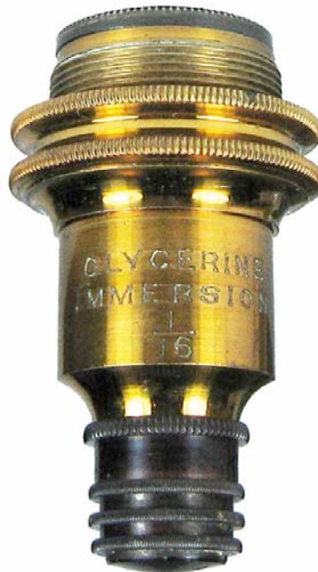
Glycerine Immersion, 1/16. c1870. Unsigned, button lenses. A glycerine immersion objective was first shown by Ernst Gundlach in Paris in 1867. 45 mm.
