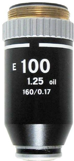
Nikon Japan, E 100, 1.25 oil, 160/0.17. c1985. The Nikon Optical Company, a Japanese firm, was established in the United States in 1953. 51mm.
