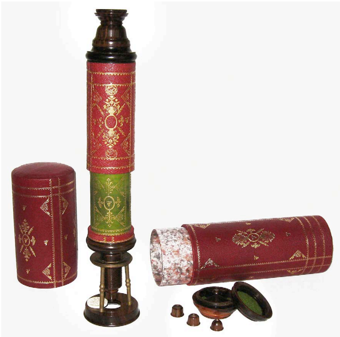
Replica of c1680 English Tripod Microscope
