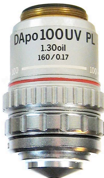
Olympus Japan, DApO 100 UV PL, 1.30oil, 160/0.17, 100, 102311. c1990. An apochromatic (Apo), 100X, ultraviolet light transmitting (UV), phase contrast positive low (PL), spring-loaded objective with iris diaphragm. A complex and versatile objective. 50mm.
