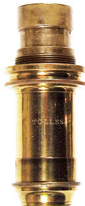
Tolles. "4 In." on canister. c1875. 4 inch continuously variable to 3 inch by internal draw-tube. Robert B. Tolles (1822-1883) apprenticed with Charles A. Spencer and supervised the Boston Optical Works from 1867 to 1883. He was renowned for his high quality objectives. 80mm extended.
