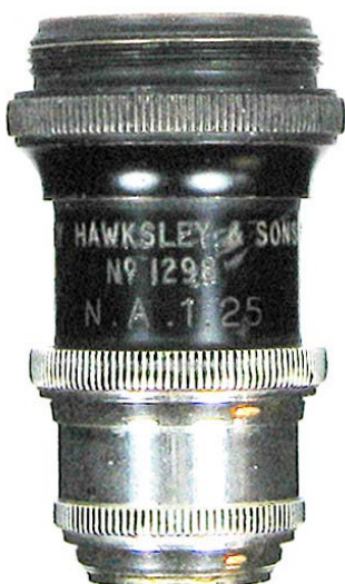
Ex d by Hawksley & Sons Ltd., 1/12, N° 1298, N.A. 1.25 Oil Immersion. c1925. Hawksley and Sons Limited, established in 1869 by Charles Hawksley, is a manufacturer of medical and laboratory equipment. 38mm.
