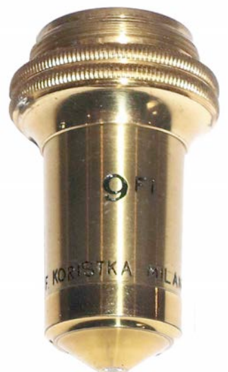
F. Koristka Milano, 9 Fl. c1920. A 1/12 fluorite objective. 40mm.
