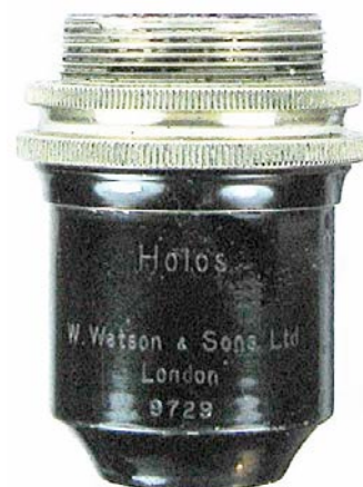
Holo, W Watson & Sons, Ltd, London, 9729, 16 mm, 45 n.a, X 10, Tube Length, 160 mm. c1950. 34 mm.
