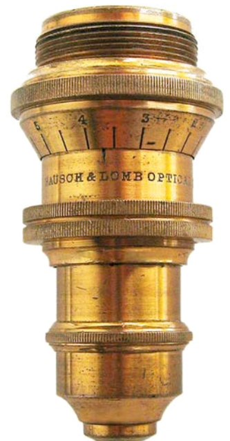
Bausch & Lomb Optical Co., 1/6, 140°. Correction collar. c1890. The Bausch & Lomb Optical Company founded by John Jacob Bausch (1830-1926) and Henry Lomb (1828-1908) began producing microscopes in 1874 in Rochester, New York. 52mm.
