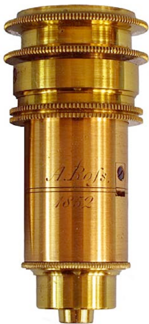
A. Rofs, 1852. Uncovered, Covered. On lid, "1/4 In. A. Rofs, London." Correction collar. One of the foremost microscope makers in London, Andrew Ross (1798-1859) began business in 1830 and collaborated with Joseph J. Lister (1786-1869) who perfected achromatic lenses. 51mm.
