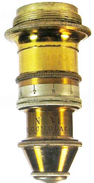
N° VI, E. Gundlach. "1/12 in" on lid. c1870. Correction collar. Ernst Gundlach worked in Berlin from 1865 to 1871 before coming to America. 49mm.
