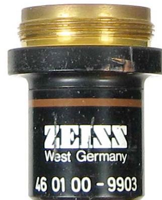
Zeiss, West Germany, 3,2/0,07, 160/-, 46 01 00 - 9903. c1970. 28 mm.
