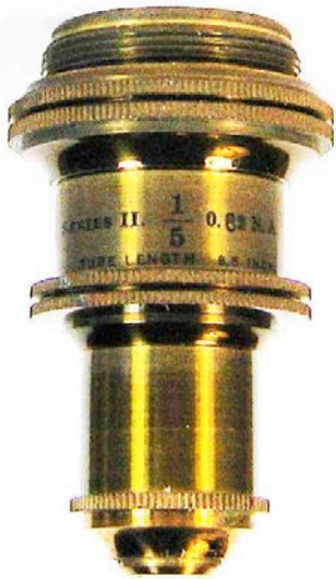
Bausch & Lomb Optical Co., Rochester N. Y. & New York City., Series II. 1/5 0.82 N. A. , Tube Length 8.5 Inch. c1895. 41mm.
