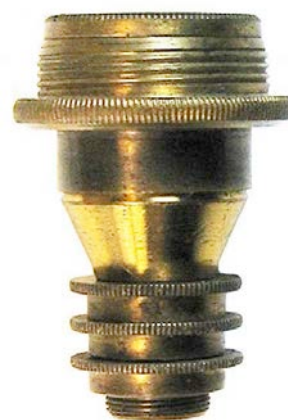
Unmarked three-element button objective with a 1/2 inch diameter thread. c1840. Objectives of this type have stackable button lenses that can be screwed on in different combinations to produce a variety of focal lengths. Frequently used on microscopes in the mid 19 th century. 25mm.
