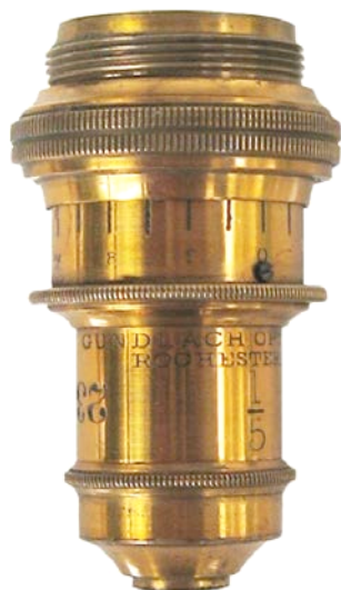
Gundlach Optical Co, Rochester N. Y., 1/5, N. A. 0.92, D, 23. Correction collar. c1890. Ernst Gundlach operated the Gundlach Optical Company in Rochester from 1884 to 1895. 44mm.
