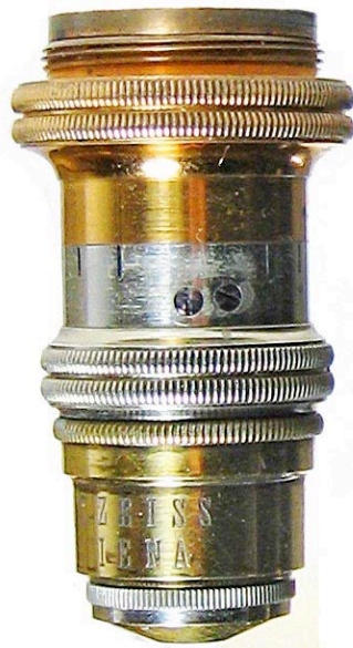
C. Zeiss, Jena, 2.5 Mm, Apert 1.25, Tubusl 160 Mm. Correction collar. Wasser Immers. and 118 on lid. c1900. 46mm.
