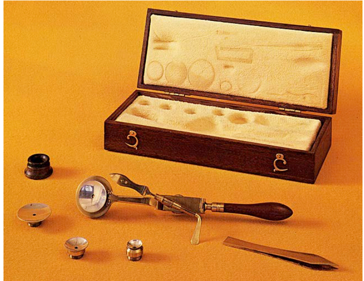
Simple Compass Microscope, Lieberkuhn Type Replica, c. 1780
