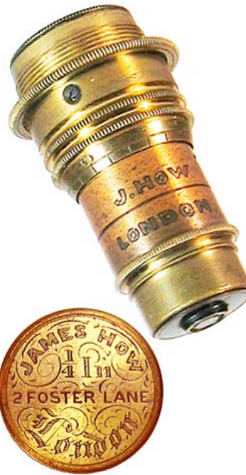
J. How., London., Uncovered., Covered. "1/4 In" on lid. Correction collar. c1870. James How operated at 2 Foster Lane from about 1860 to 1880. 46mm.
