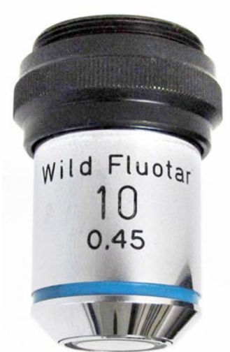
Wild Fluotar, 10, 0.45, Wild Heerbrugg Switzerland 104629. c1970. A fluorite objective. The firm of Wild Heerbrugg was established in 1921 in Switzerland and made its first microscope in 1939. 36mm.
