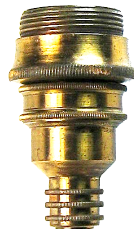
Triplet button objective with 3 screw-on lenses. Marked "1" on canister lid. c1840. Shown with adapter from objective internal female thread (0.44 in.) to male RMS thread. 27mm.
