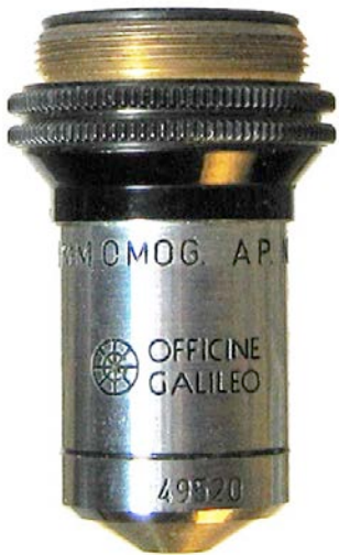
Officine Galileo, 97X, 1.8mm Imm.Omog. AP. N. 1.30, 249520 Made In Italy. c1960. Officine Galileo traces its origin to Giovanni Battista Amici (1786-1863) in 1862 in Florence, Italy. 38mm.
