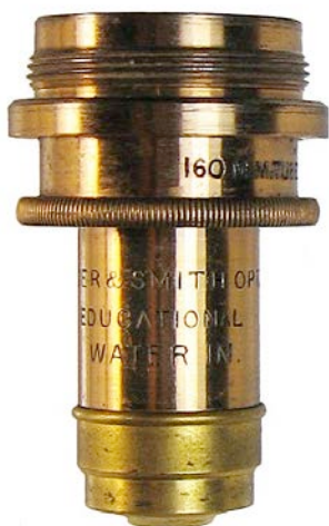
Spencer & Smith Opt. Co., Educational, Water Im., 1018, 160M.M.Tube. "1/10" on lid. Herbert R. Spencer (1849-1900) formed a partnership with Fred R. Smith and between 1890 and 1895 the firm was known as Spencer & Smith Optical Company. 37mm.
