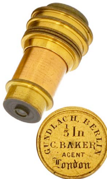
Unmarked objective. c1865. "Gundlach, Berlin, 1/5 In, C. Baker, Agent, London" on canister lid. Objective by Baker? 50mm.
