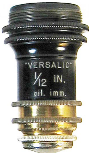
W. Watson & Sons Ltd., London, 2311, "Versalio," 1/12 IN., oil. imm. c1910. Watson & Sons Ltd. was active from 1908 to 1969. 39mm.
