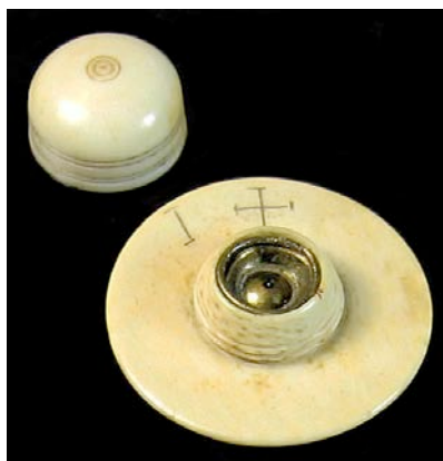
Objective for a screw barrel microscope. Ivory with cap and button lens. c1710. Closely resembles objectives made by James Wilson (1665-1730) (Clay and Court, Figs. 21, 22). Other possible makers are Edmund Culpeper (1670-1738) and Edward Scarlett (c1677-1743). 30mm wide.
