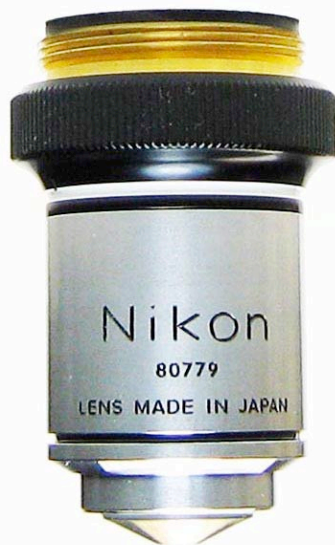
Nikon, 80779, Lens Made In Japan, s HI 100 1.25. c1980. For homogeneous immersion. 39mm.
