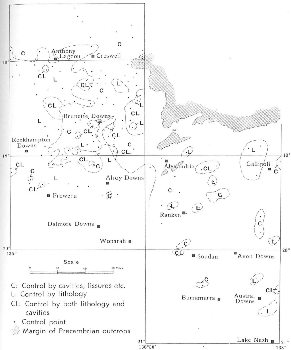
Fig. 5: Control of aquifer.
