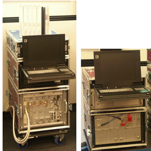
Receiver Unit and Transmitter Unit VXI design mounted in rugged portable 19" racks
