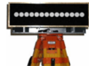
8x2 PULA Dual polarized uniform linear patch array
