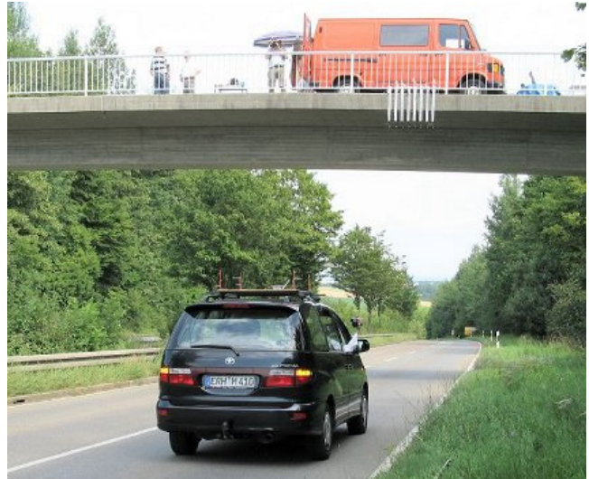
4 x 8 MIMO measurements for largely varied antenna spacing at a motorway bridge
