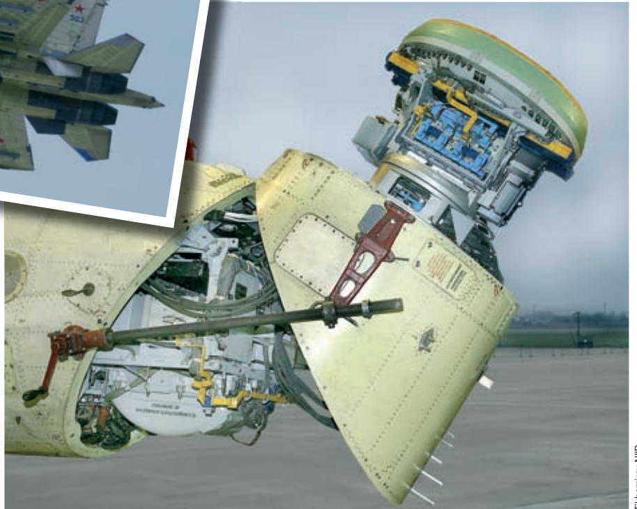
Irbis-E phased-array radar is being tested onboard the Su-30MK2 No 503 flying testbed since early 2007
