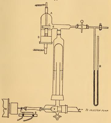
this tube as shown; the cloud on which the observations were made was formed between them, and they could be maintained at any required difference of potential up to 2000 volts by means of a battery of small secondary cells. A glass tube E was sealed on to the side of AB and served to connect the space between the disks with an apparatus for producing a sudden expansion of any desired amount. A small mercury manometer (H) was used to measure the expansion,
