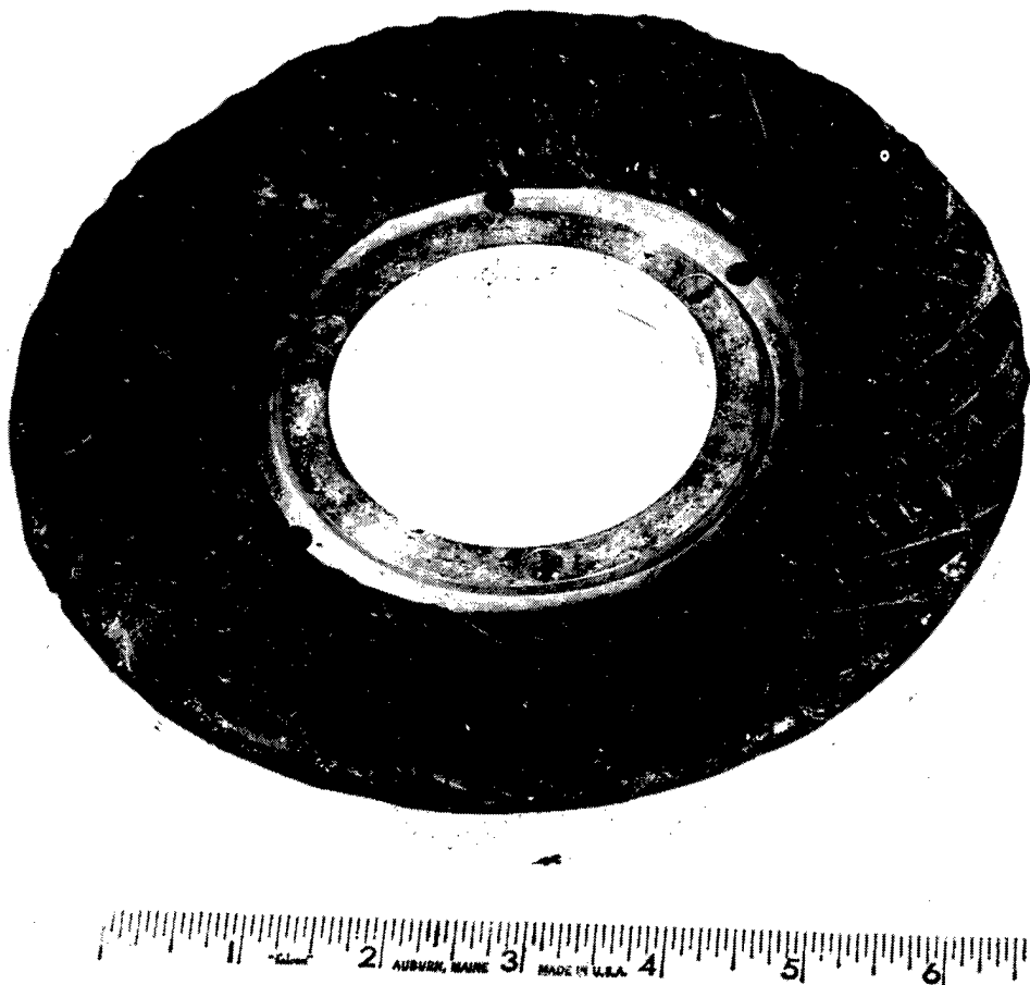
Figure 6. 7 3/4-in. rigid pitch lap used to polish 13-in. flat
