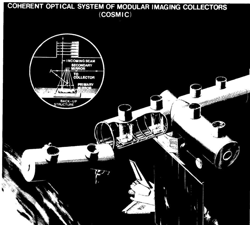
Figure 22. Assembly of a large coherent array of optical telescopes. Such arrays may be used to achieve very high angular resolution as well as to build up a large collecting area.
