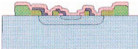
FIGURE 2072-9. Metallization misalignment, cross section view.
