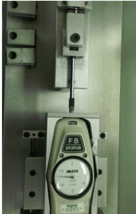
FIGURE 2038-1. Sample apparatus fixture with force measuring gauge.
