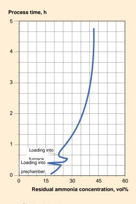
a. Obtained depths: Compound layer: 12 µm Diffusion zone: 0.24 mm
