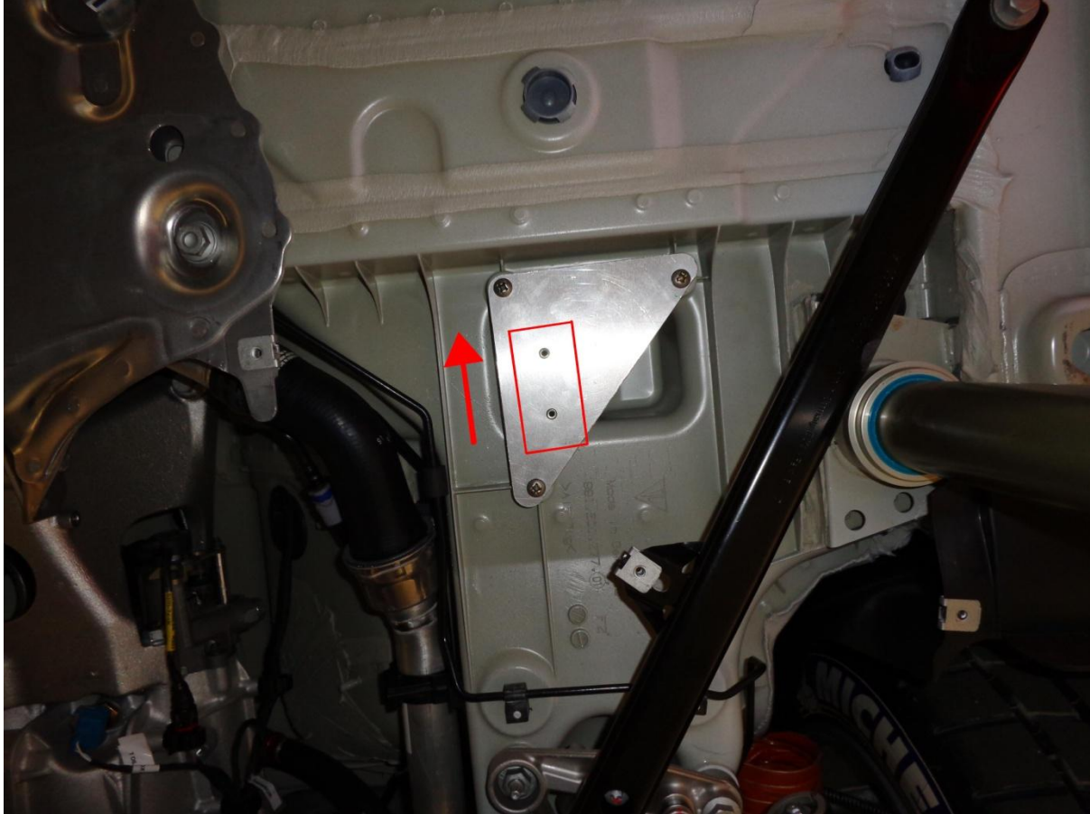
LOCATION OF DORIAN DATA 1 MICRO TIMING TRANSMITTER (FLOOR PAN REMOVED)
