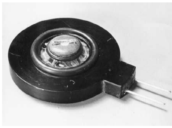
Figure 9. Prototype 'Delieu Walker' (DW) apparatus for polarographic measurement of oxygen by isolated chloroplasts etc. Above: glass chamber with plunger to exclude air and plexiglass water jacket. Below: electrode disc removed to show central platinum cathode, membrane and magnetic follower (flea).
