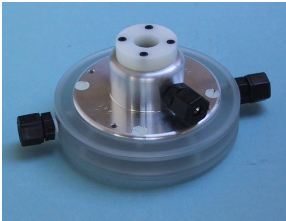
Model SG-103M laser-triggered switch for precise, low-jitter (<5 ns) operation: 10–30 kV, 50 kA, \leq 20 nH
