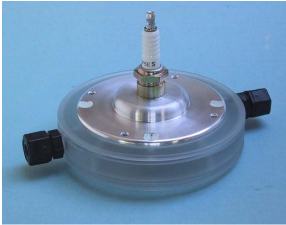
Model SG-101M trigatron (electrically triggered) switch for moderately HV applications: 10–40 kV, 100 kA, <35 nH
