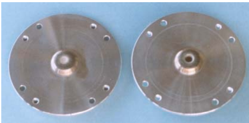
Model SG-141M trigatron switch after ~1M shots ( H_2 gas, 50-100 pps, 5-10 kV, 4-8 kA).
