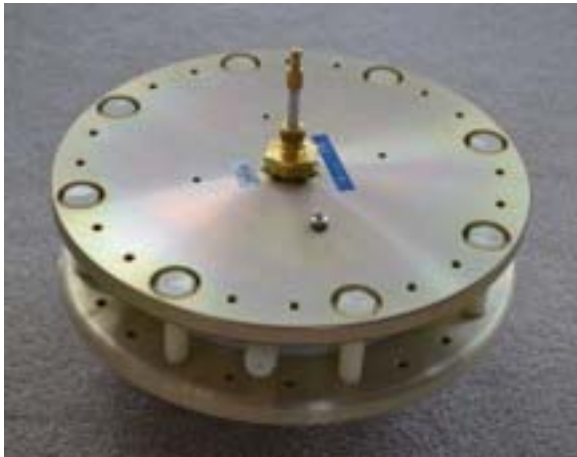
Model SG-171M trigatron switch for high-current, large charge-transfer applications: 10–35 kV, 200 kA, 5 C, \leq 35 nH
