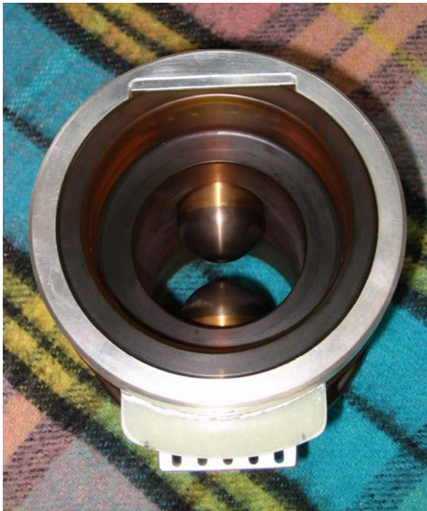
Model SG-203 photo-triggered switch for MV-1 Marx generator: 25–85 kV, 100 kA, 0.5 C
