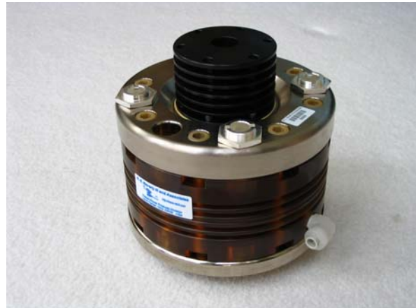
Model SG-183 field-distortion switch for direct mounting on Scyllac-style capacitors: 10–36 kV, 250 kA, 1 C, 26 nH
