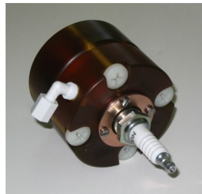
Model SG-104 demountable mini-trigatron switch: 5–40 kV, 65 kA, \approx 35 nH
