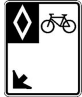
Reserved Bicycle Lane Sign
