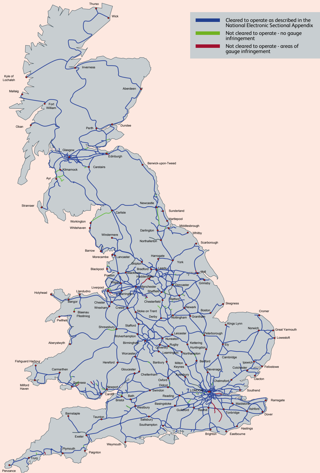
Figure 5.3 – Routes with structures with foul or special reduced clearances to a Mk 2 vehicle
