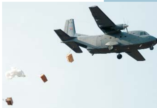
A Casa transport aircraft doing platform low extraction delivery system (PLEDS) drops.
