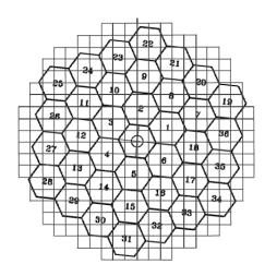
**Figure 1:** The pattern of the 36 segments (hexagons) superimposed on the subapertures of the current Keck wavefront sensors. The image on the right has a rotation of the Keck Pupil of 6 degrees with respect to the left hand image. An example of a dramatic illumination change is the subaperture at the top left side of segment 22. It goes from partial illumination to almost no illumination as the pupil rotates in the images above.
