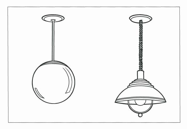
Suspended uplight/downlight luminaires provide ambient lighting. Some are made from clear or frosted glass or plastics. They are available in various sizes and shapes. They typically house incandescent lamps, although some may accommodate compact fluorescent lamps. Suspended uplight/downlight luminaires that house linear fluorescent lamps are common in commercial applications but also can be used attractively in homes.
