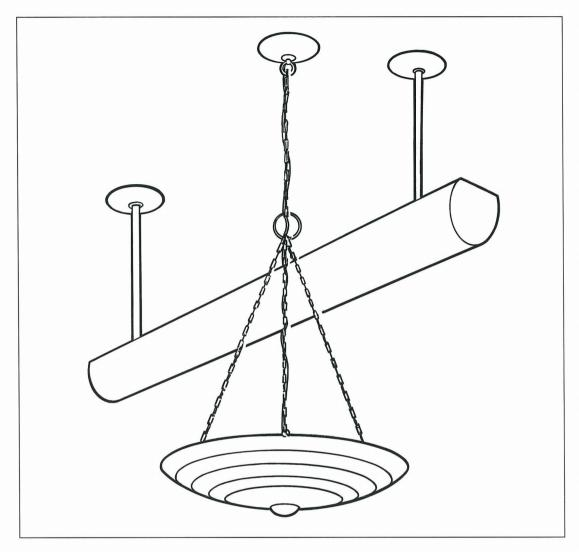
Suspended uplights direct most of the light toward the ceiling and upper portion of the walls so that these surfaces serve as reflectors. Uplights can create a soft, shadowless light in a room. Consider introducing a downlighting element to the design by using suspended uplights made of translucent materials.
