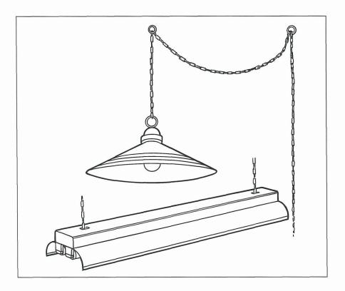
Suspended downlights direct most of the light downward. The lighting distribution patterns vary with the size and shape of the luminaire. To shield the lamps from view, luminaires that are used for ambient lighting typically have a translucent shade and those used for table lighting have an opaque metal or fabric shade. In most cases, suspended downlights used for task lighting should be supplemented with other luminaires that provide ambient lighting.
