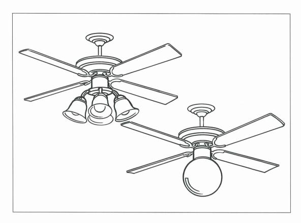
Ceiling paddle fans may include a luminaire. Many have a single globe or multiple decorative shades on arms located below the fan. Uplights are also offered with some fans. Some manufacturers offer a removable "light kit" option, which usually contains incandescent lamps.
