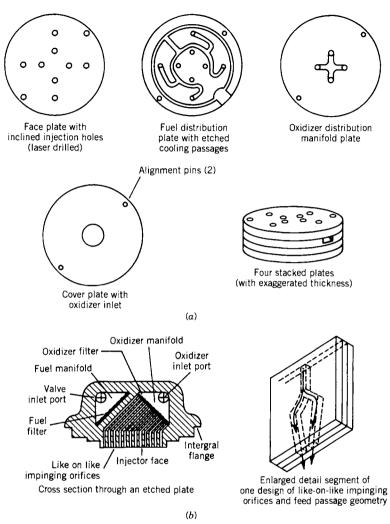
**FIGURE 8–5.** Simplified diagrams of two types of injector using a bonded platelet construction technique: (a) injector for low thrust with four impinging unlike doublet liquid streams; the individual plates are parallel to the injector face; (b) Like-on-like impinging stream injector with 144 orifices; plates are perpendicular to the injector face. (Courtesy of Aerojet Propulsion Company.)
