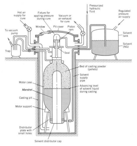
FIGURE 12–12. Simplified diagram of one system for slurry casting and initial curing of a double-base solid propellant.
