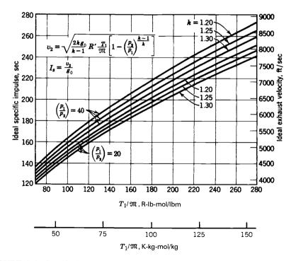
**FIGURE 3–2.** Specific impulse and exhaust velocity of an ideal rocket at optimum nozzle expansion as functions of the absolute chamber temperature  $T_1$  and the molecular mass  $\mathfrak{M}$  for several values of k and  $p_1/p_2$ .
