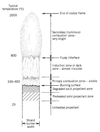
FIGURE 13–1. Schematic diagram of the combustion flame structure of a double-base propellant as seen with a strand burner in an inert atmosphere. (Adapted from Chapter 1 of Ref. 13–1 with permission of the American Institute of Aeronautics and Astronautics, AIAA.)
