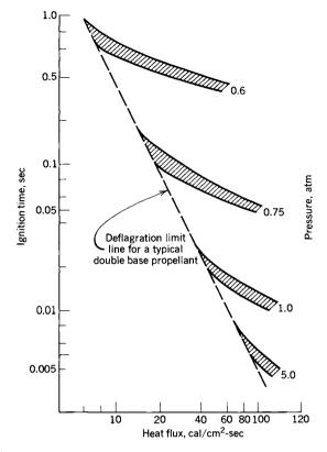
FIGURE 13-4. Propellant ignitability curves: effect of heat flux on ignition time for a specific motor.
