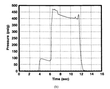
**FIGURE 15–11.** (a) An example of large-amplitude, high-frequency combustion pressure oscillations due to flame-holding instability in an 11-in. diameter GOX/HTPB motor. Instability during the initial one second of burn has been suppressed by the use of a pilot flame. (b) Suppression of flame-holding instability in an 11-in. diameter GOX/HTPB motor by means of strong axial injection of oxidizer.
