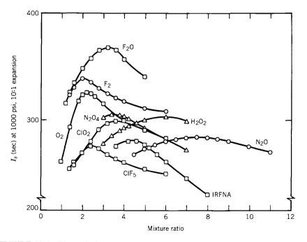
**FIGURE 15–2.** Theoretical vacuum specific impulse of selected oxidizers reacted with hydroxyl-terminated polybutadiene fuel. The  $I_s$  of the O<sub>2</sub>/HTPB propellant is comparable to that of a LOX/kerosene bipropellant engine.
