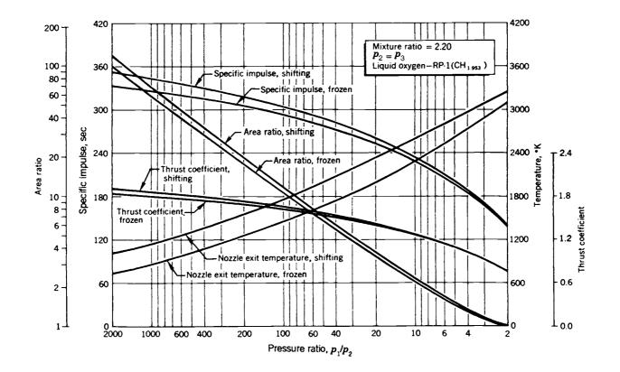
**FIGURE 5–5.** Variation of calculated parameters with pressure ratio for liquid oxygen-hydrocarbon propellant at a mixture ratio of 2.20. An increase in pressure ratio is due to an increase in chamber pressure, a decrease of nozzle exit pressure (larger area ratio and higher altitude), or both.
