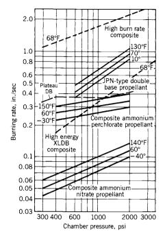
**FIGURE 11–6.** Plot of the burning rate versus chamber pressure for several typical solid rocket propellants, some at three different temperatures. A particular *double base* plateau propellant shows a constant burning rate over a fairly wide pressure range.
