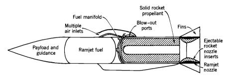
FIGURE 1-7. Elements of an air-launched missile with integral rocket-ramjet propulsion. After the solid propellant has been consumed in boosting the vehicle to flight speed, the rocket combustion chamber becomes the ramjet combustion chamber with air burning the ramjet liquid fuel.
