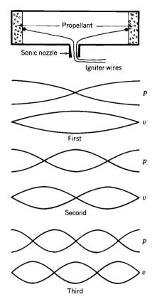
FIGURE 13-7. Standard T-burner and its longitudinal mode standing waves (pressure and velocity).
