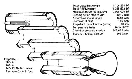
FIGURE 14-2. Simplified diagram of the four segments of the Space Shuttle solid rocket motor. Details of the thrust vector actuating mechanism or the ignition system are not shown. (Courtesy of NASA and Thiokol Propulsion, a Division of Cordant Technologies, Inc.)
