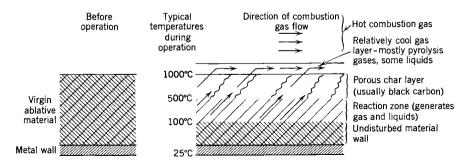
**FIGURE 14-11.** Zones in an ablative material during rocket operation with fibers at  $45^{\circ}$  to the flow.
