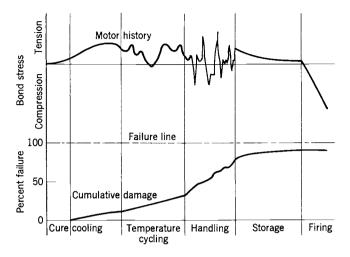
**FIGURE 11–25.** Representation of the progress in cumulative damage to the bond between the grain and the case in a case-bonded rocket motor experiencing a hypothetical stress history. (Adapted from Ref. 11–30.)
