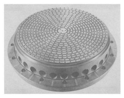
**FIGURE 8-4.** Injector with 90° self-impinging (fuel-against-fuel and oxidizer-againstoxidizer)-type countersunk doublet injection pattern. Large holes are inlets to fuel manifolds. Pre-drilled rings are brazed alternately over an annular fuel manifold or groove and a similar adjacent oxidizer manifold or groove. A section through a similar but larger injector is shown in Fig. 8–1.
