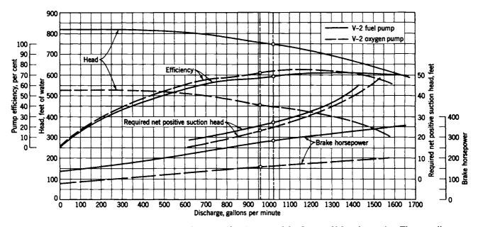
FIGURE 10-6. Water test performance curves of the centrifugal pumps of the German V-2 rocket engine. The propellants are diluted 75% ethyl alcohol and liquid oxygen.
