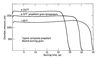
**FIGURE 11–8.** Effect of propellant temperature on burning time and chamber pressure for a particular motor. The integrated areas under the curves are proportional to the total impulse, which is the same for the three curves.
