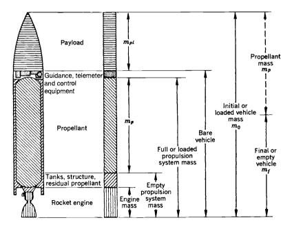
FIGURE 4-1. Definitions of various vehicle masses.
