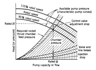
**FIGURE 10–15.** Simplified diagram of the balance of available and required feed pressures versus flow for one of the propellants in a rocket engine with a turbopump feed system. Chamber pressure is increased by liquid column.
