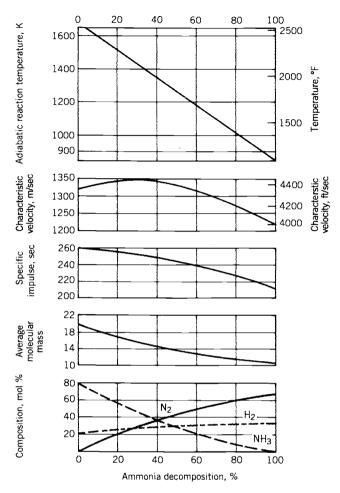
**FIGURE 7–3.** Operating parameters for decomposed hydrazine at the exit of a catalytic reactor as a function of the ammonia dissociation fraction. Adapted with permission from Ref. 7–8.
