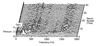
**FIGURE 9–5.** Graphical representation of a series of 40 superimposed frequencyamplitude diagrams taken 0.200 sec apart during the start phase (for the first 8 sec) of the Vulcain HM 60 thrust chamber. In this static hot-firing test the thrust chamber was operating at 109 bar chamber pressure and an oxidizer-to-fuel mass flow mixture ratio of 6.6. (Copied with permission from Ref. 9–13).
