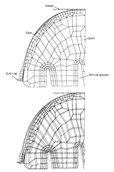
**FIGURE 11–22.** Finite element analysis grid of the forward end of a cast grain in a filament-wound plastic case. The grain has an internal tube and annular grooves. The top diagram shows the model grid elements and the bottom shows one calculated strain or deformation condition. (Reprinted with permission from A. Turchot, Chapter 10 of Ref. 11–1).
