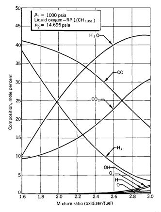
**FIGURE 5–3.** Calculated nozzle exit gas composition for shifting equilibrium conditions as a function of mixture ratio. Breakdown into O, OH, or H and free  $O_2$  occurs only at the higher temperatures or higher mixture ratios.
