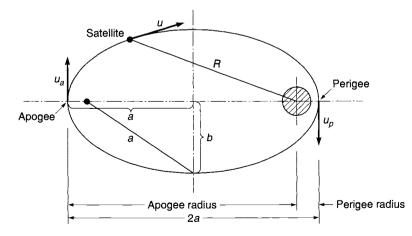
FIGURE 4-7. Elliptical orbit; the attracting body is at one of the focal points of the ellipse.
