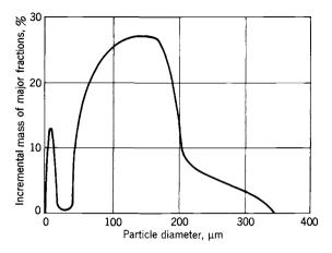
**FIGURE 12–10.** The oxidizer (AP) particle size distribution is a blend of two or more different particle sizes; this particular composite propellant consists of a narrow cut at about 10  $\mu$ m and a broad region from 50 to 200  $\mu$ m.
