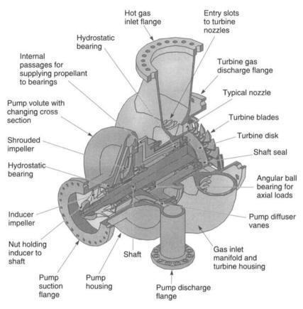
**FIGURE 10–1.** Cut-away view of an experimental turbopump demonstrator with a single-stage liquid oxygen pump impeller, an inducer impeller, and a single-stage turbine (one row of blades) on the same shaft. (Courtesy of The Boeing Company, Rocketdyne Propulsion and Power.)
