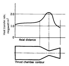
**FIGURE 8–8.** Typical axial heat transfer rate distribution for liquid propellant thrust chambers and solid propellant rocket motors. The peak is always at the nozzle throat and the lowest value is usually near the nozzle exit.
