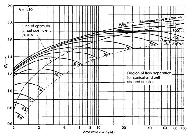
**FIGURE 3-8.** Thrust coefficient  $C_F$  versus nozzle area ratio for k = 1.30.
