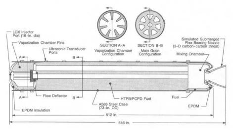
**FIGURE 15–4.** 250,000 lbf thrust hybrid booster design parameters and section of fuel grain and nozzle. The vaporization chamber fins and flow deflector are designed to promote flame holding in combustion ports.
