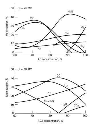
**FIGURE 12–7.** Calculated combustion products of composite propellant with varying amounts of AP or RDX. (Adapted from Chapter 1 of Ref. 12–2 with permission of the AIAA.)
