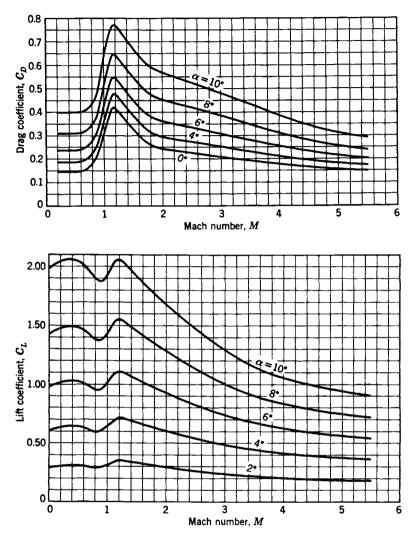
**FIGURE 4-3.** Variation of lift and drag coefficient with Mach number of the German V-2 missile based on body cross-sectional area with jet off and without exhaust plume effects at several angles of attack  $\alpha$ .
