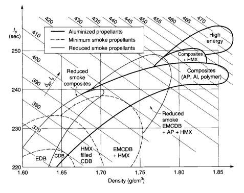
FIGURE 12-2. Estimated actual specific impulse and specific gravity for several solid propellant categories. (Adapted and reproduced from Ref. 12-1 with permission of the AIAA.)
