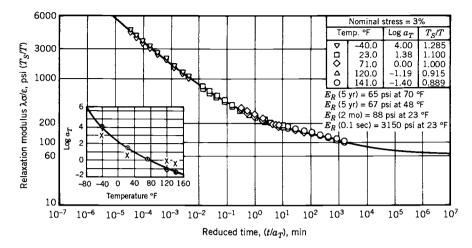
**FIGURE 11–23.** This stress-relaxation modulus master curve for a particular composite solid propellant is constructed from manipulated data taken from a number of uniaxial tensile tests at constant strain rate but different temperatures. (Reproduced with permission of United Technologies Corp., Chemical Systems from Ref. 11–27.)
