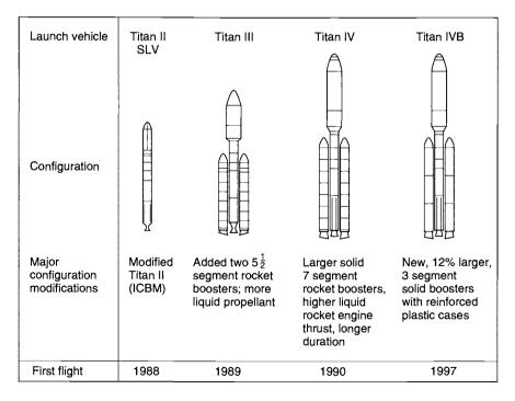
**FIGURE 4–15.** Upgrading methods are illustrated by these four related configurations in the evolution of the Titan Space Launch Vehicle family. Source: Lockheed-Martin Corp.
