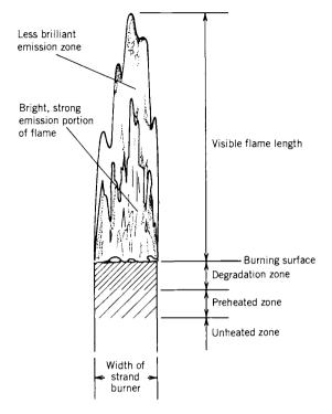
FIGURE 13–2. Diagram of the flickering, irregular combustion flame of a composite propellant (69% AP, 19% Al, plus binder and additives) in a strand burner with a neutral atmosphere. (Adapted from Chapter 1 of Ref. 13–1 with permission of AIAA.)
