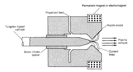
**FIGURE 19-9.** Simplified diagram of a magnetoplasma dynamic (MPD) arcjet thruster. It is similar in construction to the thermal arcjet shown in Fig. 1–8 but it has a stronger magnetic field to enhance the propellant acceleration.
