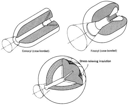
Spherical (case-bonded) with slots and cylinder
