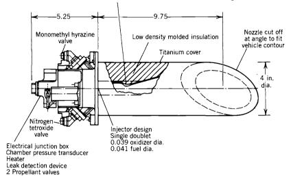
Columbium chamber with disilicide coating (0.003 in. thick)
