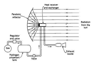
FIGURE 1-11. Simplified schematic diagram of a solar thermal rocket concept.
