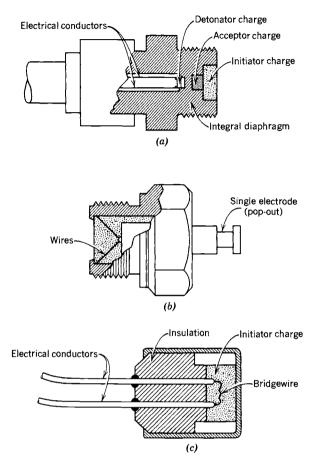
**FIGURE 14–15.** Typical electric initiators; (a) integral diaphragm type; (b) header type with double bridgewire; (c) exploding bridgewire type.
