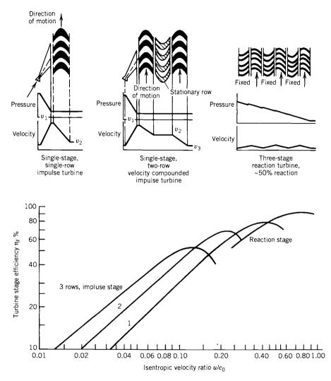
**FIGURE 10–9.** Top view diagram, pressure and velocity profiles, and efficiency curves for impulse and reaction type turbines. The velocity ratio is the pitch line velocity of the rotating blades u divided by the theoretical gas spouting velocity  $c_0$  derived from the enthalpy drop. Adapted with permission from Refs. 10–1 and 10–12.
