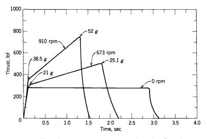
**FIGURE 11–12.** Effect of axial spin on the thrust-time behavior of a rocket motor with composite propellant using aluminum and PBAN (polybutadiene acrylonitrile) as fuels. (Adapted with permission from Ref. 11–7.)
