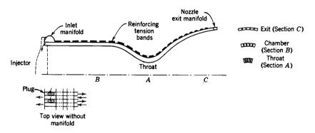
**FIGURE 8–9.** Diagram of a tubular cooling jacket. The tubes are bent to the chamber and nozzle contours; they are formed hydraulically to give a variable cross section to permit the same number of tubes at the throat and exit diameters. Coolant enters through the inlet manifold into every other tube and proceeds axially to the nozzle exit manifold, where it then enters the alternate tubes and returns axially to go directly to the injector.
