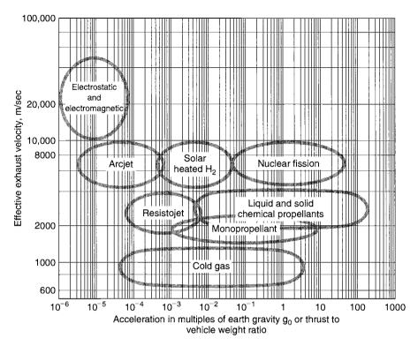
**FIGURE 2–5.** Exhaust velocities as a function of typical vehicle accelerations. Regions indicate approximate performance values for different types of propulsion systems. The mass of the vehicle includes the propulsion system, but the payload is assumed to be zero.
