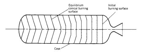
**FIGURE 11–18.** Schematic diagram of end-burning grain coning effect. In larger sizes (above approximately 0.5 m diameter) the burning surface does not remain flat and perpendicular to the motor axis, but gradually assumes a conical shape. The lines in the grain indicate successively larger-area burning surface contours.
