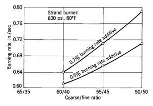
**FIGURE 12-8.** Typical effect of oxidizer (ammonium perchlorate) particle size mixture and burning rate additive on the burning rate of a composite propellant. (From NASA report SP-72262, Motor Propellant Development, July 1, 1967.)
