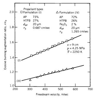
**FIGURE 11–10.** Effect of gas velocity in the perforation or grain cavity on the erosive burning augmentation factor, which is the burning rate with erosion r divided by the burning rate without erosion  $r_0$ . (Reproduced with permission of the AIAA from Chapter 10 of Ref. 11–3.)
