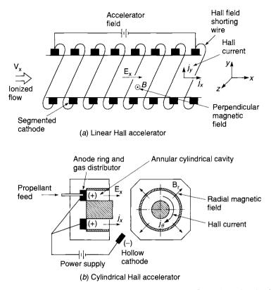
**FIGURE 19–10.** Linear and cylindrical Hall accelerator configurations showing how an applied axial field results in a transverse current that accelerates the plasma. The Hall current peaks when the external resistance is absent (i.e., shorted). The presence of any significant axial current density  $j_x$  represents an inefficiency in Hall devices.
