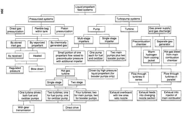
FIGURE 6-2. Design options of fed systems for liquid propellant rocket engines. The more common types are designated with a double line at the bottom of the box.
