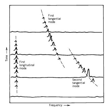
**FIGURE 13-6.** Example of mode frequency display; also called a "waterfall" diagram of a motor firing. Only four complete time-frequency curves are shown; for easy visualization the other time lines are partly omitted except near the resonating frequencies. The height of the wave is proportional to pressure. As the cavity volume increases, the frequencies of the transverse modes decrease. (Adapted from E. W. Price, Chapter 13 of Ref. 13–1, with permission of AIAA.)
