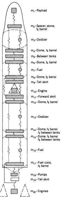
FIGURE 9-3. Typical two-stage vehicle spring-mass model used in analysis of pogo vibration in the veritcal direction.
