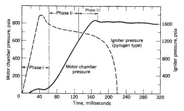
**FIGURE 13–3.** Typical ignition pressure transient portion of motor chamber pressuretime trace with igniter pressure trace and ignition process phases shown. Electric signal is received a few milliseconds before time zero.
