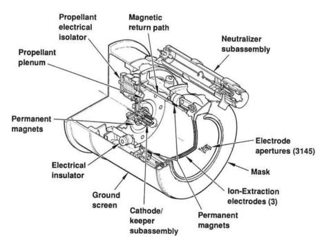
**FIGURE 19–7.** External view and section of a 500-watt ion propulsion system (XIPS), rated at 18 mN and 2800 sec. Permanent magnets are used on the outside of the ionization chamber; also shown are cathodes for ionization and for beam neutralization. Xenon gas is delivered to the ionizer, then accelerated through the three sheet electrodes, and then the ion beam is neutralized. (Drawing courtesy of Hughes Space and Communications and the American Physical Society.)
