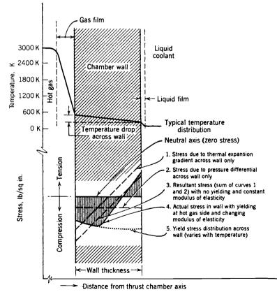
FIGURE 8-12. Typical stresses in a thrust chamber inner wall.
