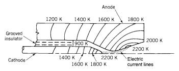
FIGURE 19-5. Typical estimated temperature distribution in the electrodes of an arcjet.
