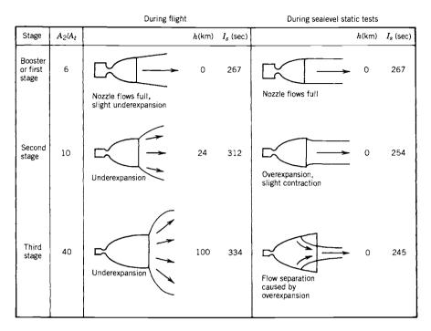
**FIGURE 3-11.** Simplified sketches of exhaust gas behavior of three typical rocket nozzles for a three-stage launch vehicle. The first vehicle stage has the biggest chamber and the highest thrust but the lowest nozzle area ratio, and the top or third stage usually has the lower thrust but the highest nozzle area ratio.
