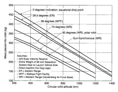
**FIGURE 4–16.** Decrease of payload with circular orbit altitude and orbit inclination for the Pegasus launch vehicle. This is an air-launched, relatively simple, three-stage launch vehicle of 50 in. diameter driven by a solid propellant rocket motor in each stage. (Courtesy Orbital Sciences Corporation)
