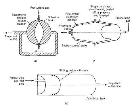
**FIGURE 6-7.** Three concepts of propellant tanks with positive expulsion: (a) inflatable dual bladder; (b) rolling, peeling diaphragm; (c) sliding piston. As the propellant volume expands or contracts with changes in ambient temperature, the piston or diaphragm will also move slightly and the ullage volume will change during storage.
