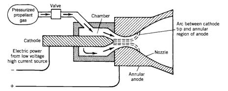
**FIGURE 1-8.** Simplified schematic diagram of arc-heating electric rocket propulsion system. The arc plasma temperature is very high (perhaps 15,000 K) and the anode, cathode, and chamber will get hot (1000 K) due to heat transfer.
