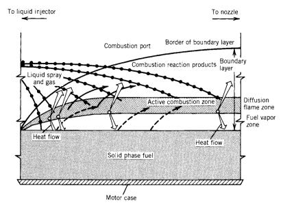
FIGURE 15–7. Simplified model of the diffusion-controlled hybrid combustion process, illustrating the flame zone embedded within the fuel boundary layer.
