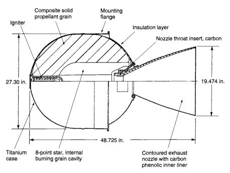
**FIGURE 11–1.** Cross section of the STAR<sup>TM</sup> 27 rocket motor, which has been used for orbit and satellite maneuvers. It has an altitude thrust of 6000 lbf, nominally burns for 34.4 sec and has an initial mass of 796 lbm. For more data see Table 11–3. (Courtesy of Thiokol Propulsion, a Division of Cordant Technologies.)
