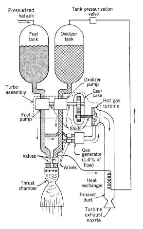
**FIGURE 1-4.** Simplified schematic diagram of one type of liquid propellant rocket engine with a turbopump feed system and a separate gas generator, which generates warm gas for driving the turbine. Not shown are components necessary for controlling the operation, filling, venting, draining, or flushing out propellants, filters or sensors. The turbopump assembly consists of two propellant pumps, a gear case, and a high speed turbine.
