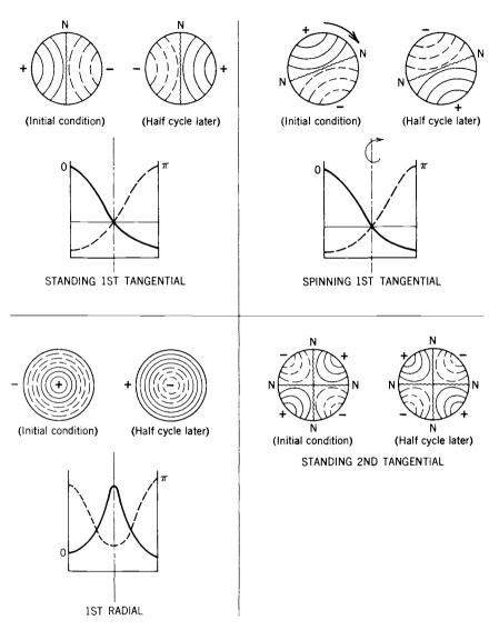
**FIGURE 9–4.** Simplified representation of transverse pressure oscillation modes at two time intervals in a cylindrical combustion chamber. The solid line curves indicate pressures greater than the normal or mean operating pressure and the dashed lines indicate lower pressures. The N–N lines show the node locations for these wave modes.
