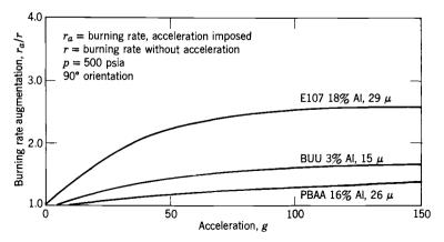
**FIGURE 11–11.** Acceleration effect on burning rate for three different propellants. (Adapted with permission from Ref. 11–7.)
