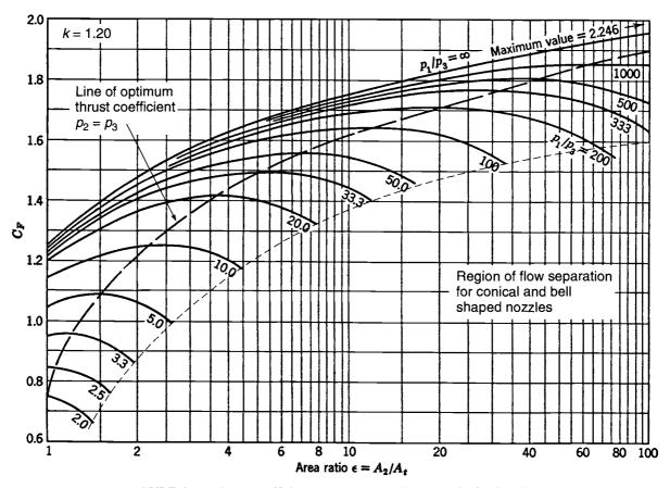
**FIGURE 3-7.** Thrust coefficient  $C_F$  versus nozzle area ratio for k = 1.20.
