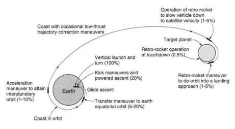
**FIGURE 4–10.** Schematic diagram of typical powered flight maneuvers during a hypothetical interplanetary mission with a landing. The numbers indicate typical thrust magnitudes of the maneuvers in percent of launch takeoff thrust. This is not drawn to scale. Heavy lines show powered flight segments.
