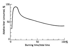
FIGURE 8-10. Relative depth of pyrolysis of ablative material with different duty cycles using many short-duration thrust pulses for a small liquid propellant reaction control thrust chamber of 20 lbf thrust.
