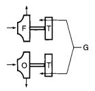
Two turbines, each with one pump. Gas flow shown in parallel. (alternate is gas flow in series, first through one and then the other turbine).
