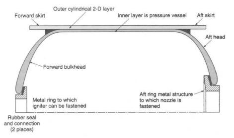
FIGURE 14-4. Simplified half-section of a typical design of a filament-wound composite material case. Elastomeric adhesives are shown in black. The outer layer reinforces the cylinder portion and provides attachment skirts. The thickness of the inner case increases at smaller diameter.
