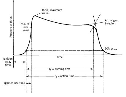
FIGURE 11-13. Definitions of burning time and action time.
