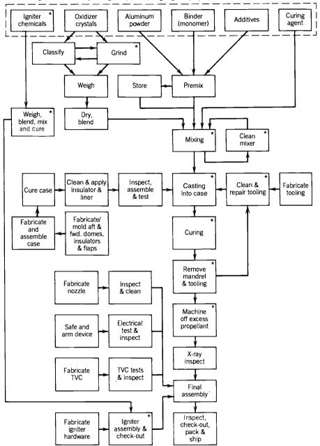
Chemical ingredients receiving, storage, inspection, weighing and preparation
