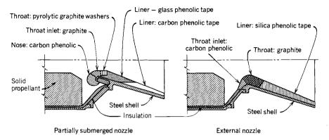
**FIGURE 14–7.** Nozzle designs for small solid propellant motors employ ablative heat sink wall pieces and graphite throat inserts resistant to high temperatures, erosion, and oxidation. The pyrolytic washers or disks are so oriented that their high conductivity direction is perpendicular to the nozzle axis.
