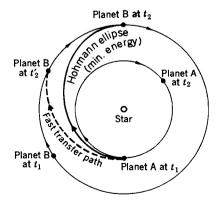
FIGURE 4–8. Schematic diagram of interplanetary transfer paths. These same transfer maneuvers apply when going from a low-altitude earth satellite orbit to a higher orbit.
