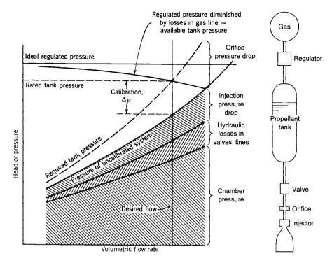
**FIGURE 10–14.** Simplified flow diagram and balance curves for the fuel or the oxidizer of a typical gas-pressurized bipropellant feed system. This diagram is also the same for a monopropellant feed system, except that it has no calibration orifice; it is calibrated by setting the proper regulated pressure.
