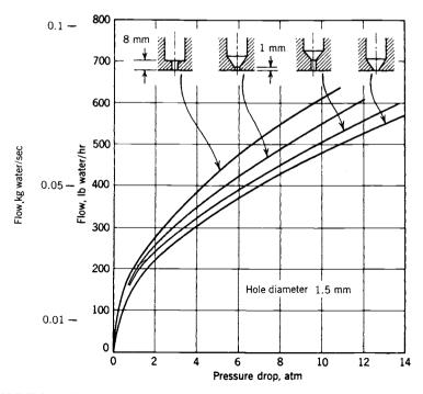
FIGURE 8-6. Hydraulic characteristics of four types of injection orifice.
