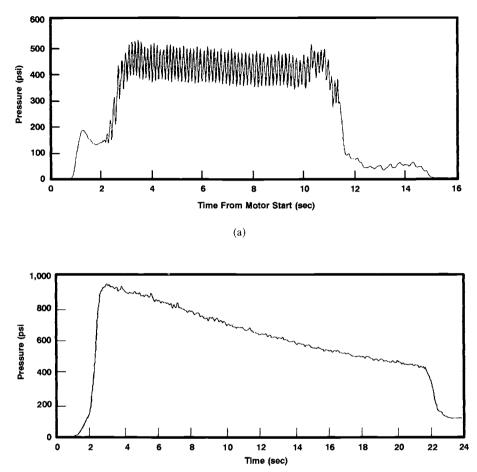
FIGURE 15–10. (a) Periodic, large-amplitude, low-frequency combustion pressure oscillations are an example of oxidizer feed system induced "chug" type combustion instability in a 24-in. diameter LOX/HTBP motor. (b) An example of stable combustion in a 24-in. diameter LOX/HTPB motor, exhibiting an overall combustion roughness level of 1.3%.
