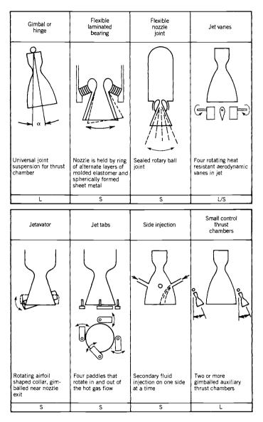
FIGURE 16-3. Simple schematic diagrams of eight different TVC mechanisms. Actuators and structural details are not shown. The letter L means it is used with liquid propellant rocket engines and S means it is used with solid propellant motors.
