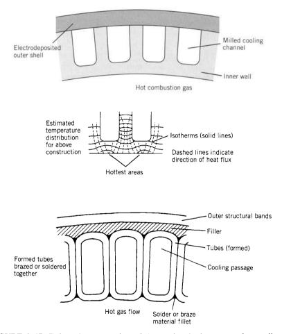
FIGURE 8-17. Enlarged cross section of thrust chamber's regenerative cooling passages for two types of design.
