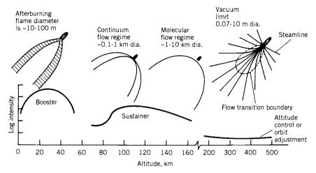
**FIGURE 18–4.** For a multistage ascending vehicle the plume radiation intensity will vary with the altitude, thrust or mass flow, propellant combination, and plume temperature. The four sketches describing the plume are not drawn to the same scale.
