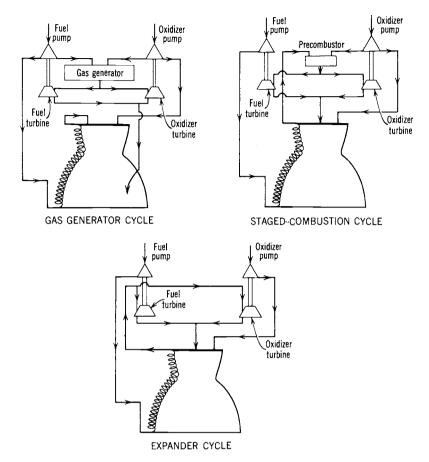
**FIGURE 6-9.** Simplified diagrams of three engine cycles for liquid propellant rocket engines. The spirals are a symbol for an axisymmetric cooling jacket where heat is absorbed.
