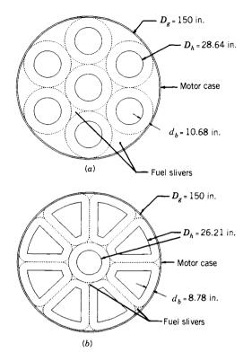
FIGURE 15-9. (a) Circular fuel grain combustion ports are volumetrically inefficient and leave large slivers at burnout. (b) Quadrilateral port hybrid grain configuration minimizes residual fuel sliver at burnout.
