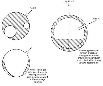
FIGURE 6-6. Ullage bubbles can float around in a zero-gravity environment; surface tension device can keep tank outlet covered with liquid.
