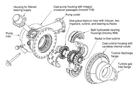
**FIGURE 10–2.** Exploded view of an advanced high-speed, two-stage liquid hydrogen fuel pump driven by a radial flow turbine. (Copied with permission of Pratt & Whitney, a division of United Technologies; adapted from Ref. 10–2.)
