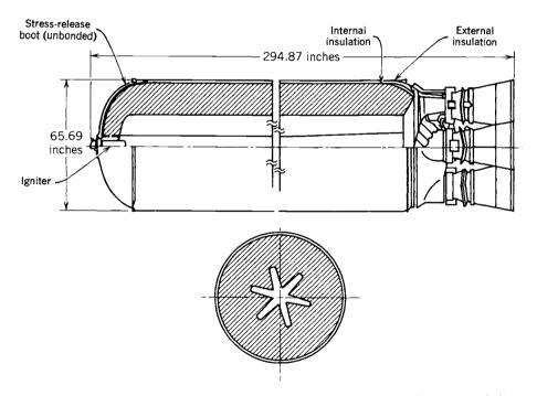
**FIGURE 16–9.** Simplified view of an early version of the first-stage Minuteman missile motor using composite-type propellant bonded to the motor case. Four movable nozzles provide pitch, yaw, and roll control. (Source: U.S. Air Force.)
