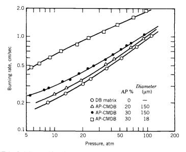
**FIGURE 11–7.** Measured burning rate characteristics of a double-base (DB) propellant and three composite-modified double-base (CMDB) propellants which contain an increasing percentage of small diameter (159  $\mu$ m) particles of ammonium perchlorate (AP). When the size of the AP particles is reduced or the percentage of AP is increased, an increase in burning rate is observed. None of these data form straight lines. (Reproduced with permission of the AIAA from Chapter 1 of Ref. 11–3.)
