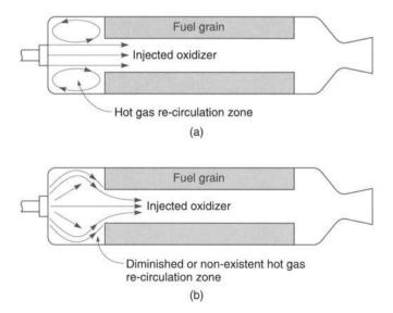
**FIGURE 15–13.** (a) Axial injection of oxidizer results in a strong hot gas flow recirculation zone at the fuel grain leading edge, producing stable combustion. (b) Conical injection of oxidizer can produce a weak or nonexistent hot gas flow recirculation zone at the fuel grain leading edge, resulting in unstable combustion.
