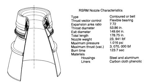
FIGURE 14-8. External quarter section view of nozzle configuration of the Space Shuttle reusable solid rocket motor (RSRM). (Courtesy of Thiokol Propulsion, a Division of Cordant Technologies.)
