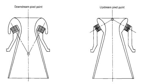
**FIGURE 16-4.** Two methods of using flexible nozzle bearings with different locations for the center of rotation. The bearing support ring is made of metal or plastic sheet shims formed into rings with spherical contours (white) bonded together by layers of molded elastomer or rubber (black stripes). Although only five elastomeric layers are shown for clarity, many flexible bearings have 10 to 20 layers. (Copied with permission from Ref. 16–1.)
