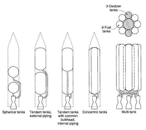
FIGURE 6-5. Typical tank arrangements for large turbopump-fed liquid propellant rocket engines.
