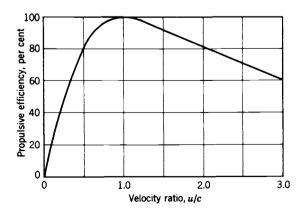
FIGURE 2-4. Propulsive efficiency at varying velocities.
