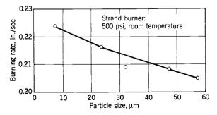
**FIGURE 12–9.** Typical effect of aluminum particle size on propellant burning rate for a composite propellant. (From NASA Report 8075, Solid Propellant Processing Factors in Rocket Motor Design, October 1971.)
