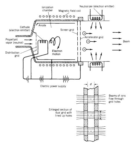
FIGURE 19–6. Simplified schematic diagram of an electron bombardment ion thruster, showing an enlarged section of the double grid.
