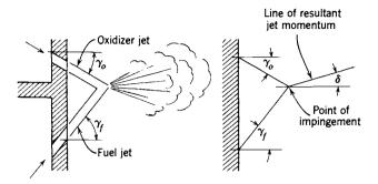
FIGURE 8-7. Angular relation of doublet impinging-stream injection pattern.
