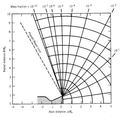
**FIGURE 18–3.** Density profile for vacuum plume expansion using a one-dimensional flow model for a small storable bipropellant thruster. The axial distance x and the plume radius R have been normalized with the nozzle exit radius  $R_e$ . Here k = 1.25, the Mach number of the nozzle exit is 4.0, and the nozzle cone half angle is 19°.
