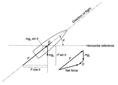
**FIGURE 4-5.** Simplified free-body force diagram for vehicle without wings or fins. The force vector diagram shows the net force on the vehicle.
