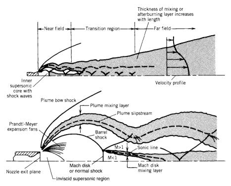
**FIGURE 18–1.** Half sections of schematic diagrams of a rocket exhaust plume at low altitude. Upper sketch shows full plume and lower sketch is an enlargement of the near field. (Reprinted with permission from Ref. 18–1.)
