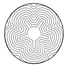
**FIGURE 11–5.** Diagram of successive burning surface contours, each a fixed small time apart. It shows the growth of the internal cavity. The lengths of these contour lines are roughly the same (within  $\pm 15\%$ ), which means that the burning area is roughly constant.
