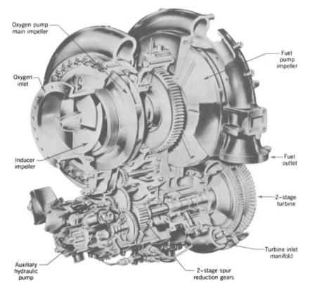
**FIGURE 10–3.** Typical geared turbopump assembly used on the RS-27 engine (Delta I and II Launch Vehicles) with liquid oxygen and RP-1 propellants. (Courtesy of The Boeing Company, Rocketdyne Propulsion and Power.)
