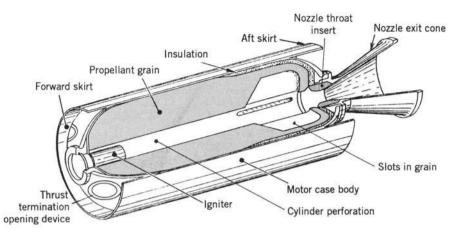
**FIGURE 1-5.** Simplified perspective three-quarter section of a typical solid propellant rocket motor with the propellant grain bonded to the case and the insulation layer and with a conical exhaust nozzle. The cylindrical case with its forward and aft hemispherical domes form a pressure vessel to contain the combustion chamber pressure. Adapted with permission from Reference 11–1.
