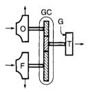
With gear case, turbine can run faster. The two pumps have different speeds.
