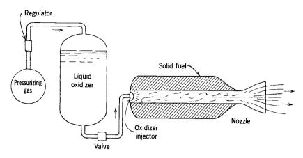
FIGURE 1-6. Simplified schematic diagram of a typical hybrid rocket engine. The relative positions of the oxidizer tank, high pressure gas tank, and the fuel chamber with its nozzle depend on the particular vehicle design.
