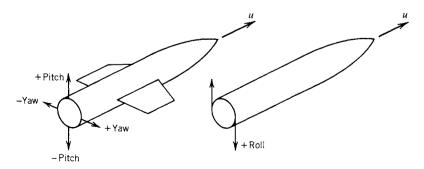
FIGURE 16-1. Moments applied to a flying vehicle.
