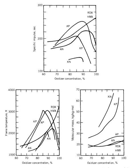
**FIGURE 12–3.** Variation of combustion temperature, average molecular mass of the combustion gases, and theoretical specific impulse (at frozen equilibrium) as a function of oxidizer concentration for HTPB-based composite propellants. Data are for a chamber pressure of 68 atm and nozzle exit pressure of 1.0 atm. (Reproduced from Ref. 12–2 with permission of the AIAA.)
