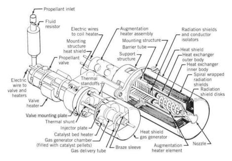
**FIGURE 19–4.** Resistojet augmented by hot gas from catalytically decomposed hydrazine; two main assemblies are present: (1) a small catalyst bed with its electromagnetically operated propellant valve and heaters to prevent hydrazine from freezing, and (2) an electrical resistance spiral-shaped heater surrounded by thin radiation shields, a refractory metal exhaust nozzle, and high-temperature electrical insulation supporting the power leads. (Courtesy of PRIMEX Aerospace Company.)
