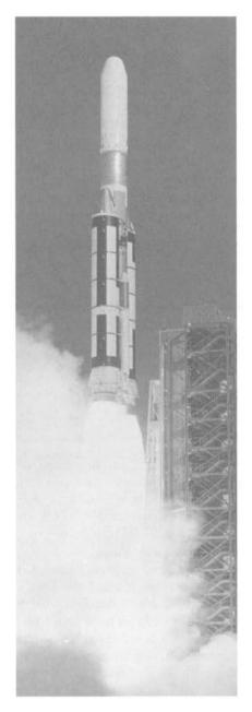
**FIGURE 1–12.** Titan III launch vehicle shortly after lift-off, with bright radiant exhaust gas. Two solid propellant rocket motors, each providing about 2.4 million pounds of thrust, boost the first stage, which also gets a sustained thrust of 470,000 pounds from two liquid rocket engines. The second stage has 100,000 pounds of thrust from a single liquid rocket engine, and one version of the third stage has two liquid rocket engines, each at 16,000 pounds of thrust.
