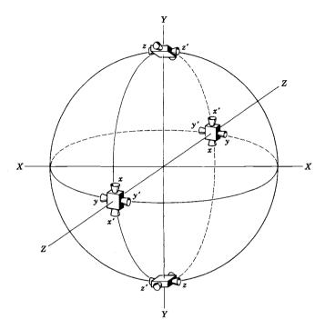
**FIGURE 4–13.** Simplified attitude control system diagram for spacecraft. It requires 12 thrusters (identified as x, y, z) to allow the application of pure torques about three perpendicular axes. The four unlabeled thrusters are needed for translation maneuvers along the z axis. They are shown here in four clusters.
