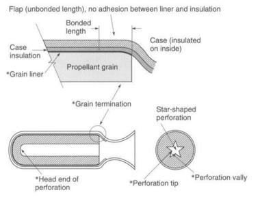
**FIGURE 11–24.** The asterisks in the bottom simplified diagram denote potentially critical failure areas. The top sketch is an enlargement of the aft termination region of the grain and shows a boot or stress relief flap.
