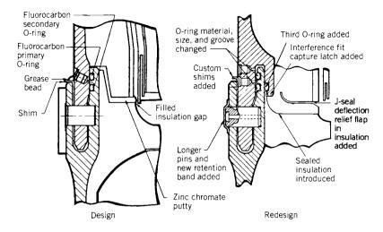
**FIGURE 14-3.** The joints between segments of the Shuttle solid rocket booster (SRB) were redesigned after a dramatic failure. The improvements were not only in a third O-ring, the mechanical joint, and its locking mechanism, but also featured a redesign of the insulation between propellant segments. (Courtesy of NASA.)
