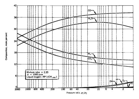
**FIGURE 5-6.** Variation of exhaust gas composition at nozzle exit with pressure ratio at a fixed mixture ratio and for shifting equilibrium. For frozen equilibrium the composition would be the same as in the chamber, as shown in Fig. 5–2.
