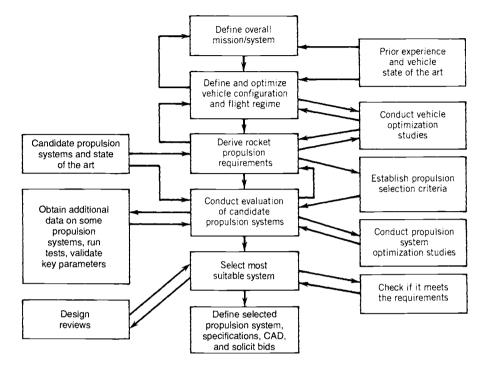
FIGURE 17-1. Idealized process for selecting propulsion systems.
