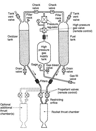
**FIGURE 1–3.** Schematic flow diagram of a liquid propellant rocket engine with a gas pressure feed system. The dashed lines show a second thrust chamber, but some engines have more than a dozen thrust chambers supplied by the same feed system. Also shown are components needed for start and stop, controlling tank pressure, filling propellants and pressurizing gas, draining or flushing out remaining propellants, tank pressure relief or venting, and several sensors.
