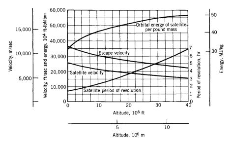
**FIGURE 4–6.** Orbital energy, orbital velocity, period of revolution, and earth escape velocity of a space vehicle as a function of altitude for circular satellite orbits. It is based on a spherical earth and neglects the earth's rotation and atmospheric drag.
