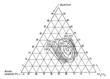
FIGURE 12-4. Composition diagram of calculated specific impulse for an ammonium perchlorate-aluminum-polyurethane (PU is a polyester binder) at standard conditions (1000 psi and expansion to 14.7 psi). The maximum value of specific impulse occurs at about 11% PU, 72% AP, and 17% Al. (Reproduced from Ref. 12-3 with permission of the American Chemical Society.)
