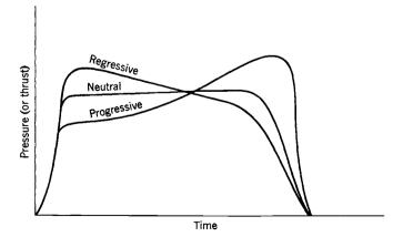
FIGURE 11-15. Classification of grains according to their pressure-time characteristics.
