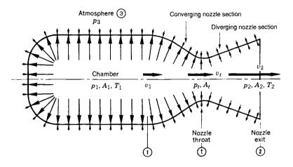
**FIGURE 2-1.** Pressure balance on chamber and nozzle interior walls is not uniform. The internal gas pressure (indicated by length of arrows) is highest in the chamber  $(p_1)$  and decreases steadily in the nozzle until it reaches the nozzle exit pressure  $p_2$ . The external or atmospheric pressure  $p_3$  is uniform. At the throat the pressure is  $p_t$ . The four subscripts (shown inside circles) refer to the quantities A, v, T, and p at specific locations.
