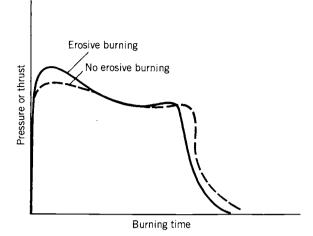
FIGURE 11-9. Typical pressure-time curve with and without erosive burning.
