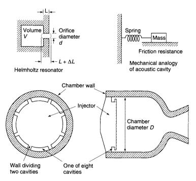
**FIGURE 9–7.** Diagram of acoustic energy absorber cavities at the periphery of an injector. In this thrust chamber the cavity restriction is a slot (in the shape of sections of a circular arc) and not a hole. Details of the chamber cooling channels, injector holes, or internal feed passages are not shown.
