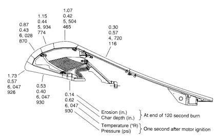
**FIGURE 14–10.** Erosion measurements and char depth data of the carbon fiber phenolic material of the nozzle of the Space Shuttle reusable solid rocket motor. (Courtesy of Thiokol Propulsion, a Division of Cordant Technologies.)
