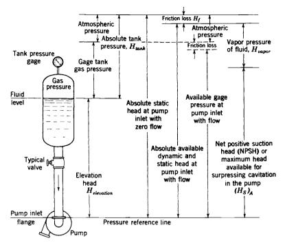
FIGURE 10-7. Definition of pump suction head.
