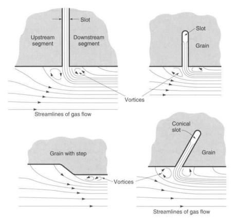
**FIGURE 13-8.** Simple sketches of four partial grain sections each with a slot or a step. Heavy lines identify the burning surfaces. The flow patterns cause the formation of vortices. The shedding of these vortices can induce flow oscillations and pressure instabilities.
