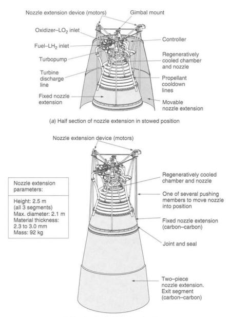
(b) Nozzle extension in deployed position
