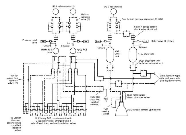
**FIGURE 6-4.** Simplified flow diagram of the propellant feed system flow for the left aft pod of the Orbital Maneuvering System (OMS) and Reaction Control System (RCS) of the Space Shuttle Orbiter Vehicle. Solid lines: nitrogen tetroxide  $(N_2O_4)$ ; dash-dot lines: monomethylhydrazine (MMH); short dashed lines: high-pressure helium. (Source: NASA.)
