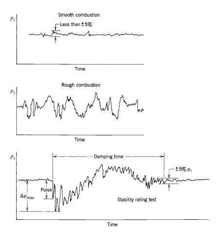
**FIGURE 9–2.** Typical oscillogrpah traces of chamber pressure  $p_1$  with time for different combustion events.
