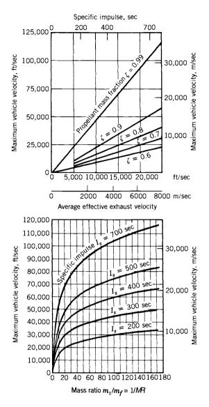
**FIGURE 4–2.** Maximum vehicle velocity in a gravitationless, drag-free space for different mass ratios and specific impulses (plot of Eq. 4–6). Single-state vehicles can have values of 1/**MR** up to about 20 and multistage vehicles can exceed 200.
