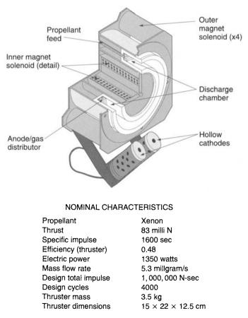
FIGURE 19-11. External view and quarter section of a 1350-watt Hall accelerator (SPT). It is rated at a thrust of 83 mN and a specific impulse of 1600 sec. The radial magnetic field is produced by an inner solenoid and four external solenoids. Ionization takes place at the beginning of the insulated annular channel. The accompanying table lists the nominal characteristics of SPT-100. (Drawing courtesy of Atlantic Research Corporation and FAKEL.)
