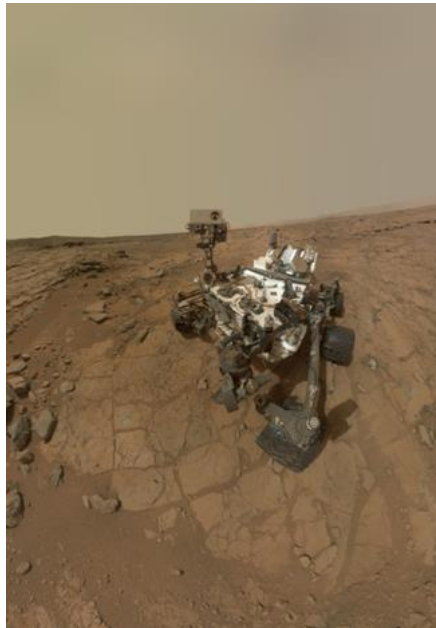
MSL Curiosity rover at "John Klein" drill site. This self-portrait of NASA's Mars rover Curiosity combines dozens of exposures taken by the rover's Mars Hand Lens Imager on Feb. 3, 2013 plus three exposures taken May 10, 2013 to show two holes (in lower left quadrant) where Curiosity used its drill on the rock target "John Klein". Credit: NASA/JPL-Caltech/MSSS
