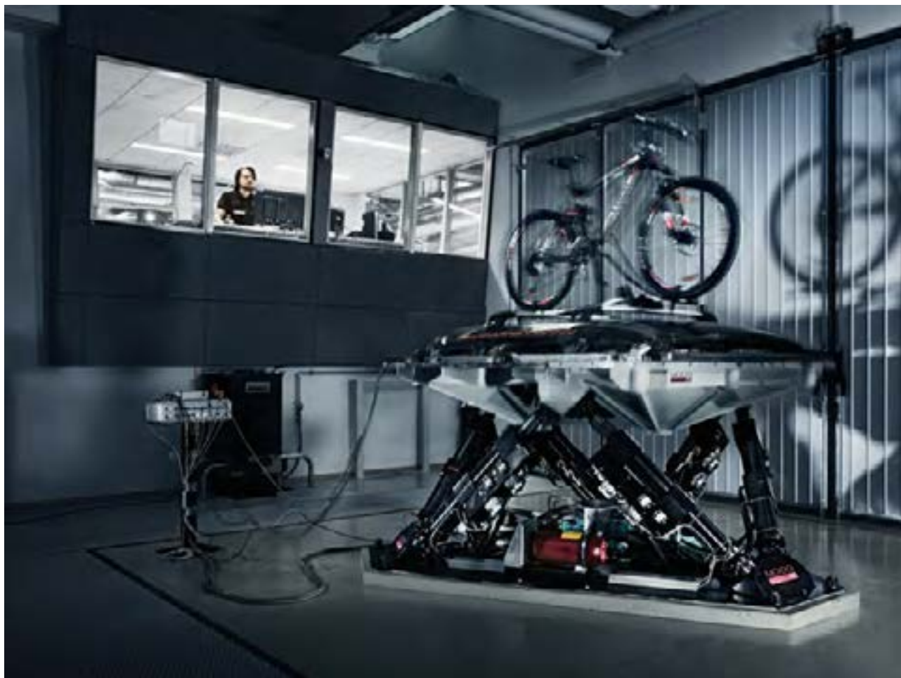
Durability and fatigue testing at Thule Test Center in Hillerstorp, Sweden
