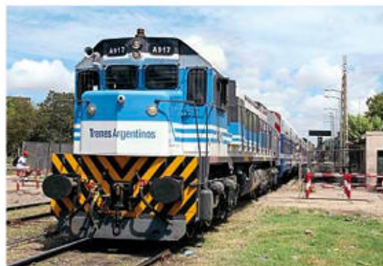
EMD-built GT22CW Co-Co A917 (built EMD, London, Canada 1998), in new Trenes Argentinos livery, departs from Florencio Varela station, working train 2237, the 11.28 Temperley-Gutiérrez on February 16. Masts for the planned electrification (this is one of the two routes to La Plata) can be seen in the picture. New EMUs will replace diesel locos on this route within a few years. D LANGHAM
