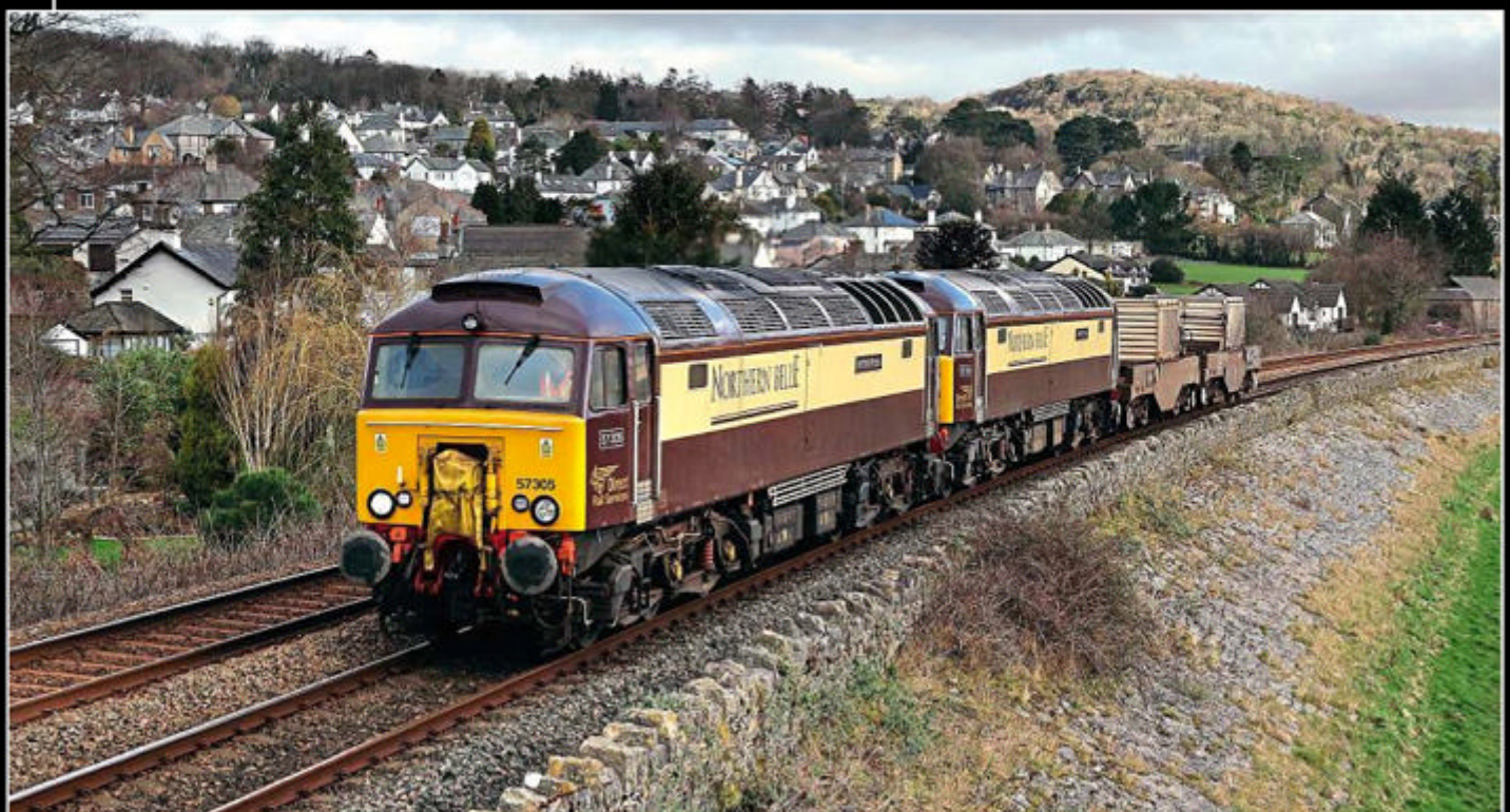
Unusual traction for the Crewe to Sellafield nuclear duty on March 22 with 'Northern Belle' Class 57s Nos. 57305 Northern Princess and 57312 Solway Princess passing Kent's Bank with two flasks in tow. TOM McATEE
