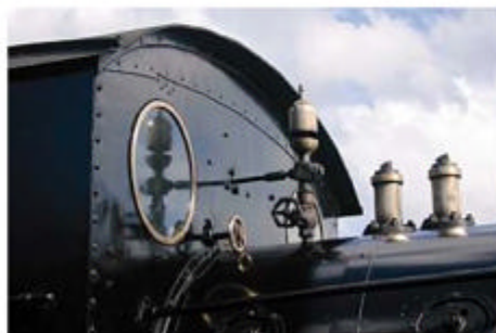
Before: The LNER-era heightened cab roof and Ross Pop safety valves. BEN BOGGIS
