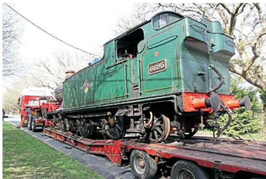
The drooping middle wheelset is evident as No. 6695 awaits recovery. ANDREW P M WRIGHT
