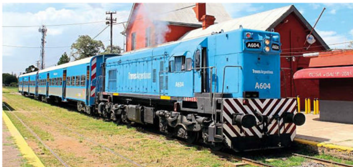
Amazingly, 1950s-built EMD G12s have replaced more recent diesel traction (including some 1980s-built three-car DMUs from Argentine firm Materfer) on some suburban services. Two daily diagrams are required for the Victoria to Capilla del Señor line, north of Buenos Aires, with four G12s dedicated to the service. On February 18, A604, in the new Trenes Argentinos livery, first delivered to Argentina in 1957, makes a smoky departure from Garin, while working train 2007 the 10.48 Victoria-Capilla del Señor. D LANGHAM
