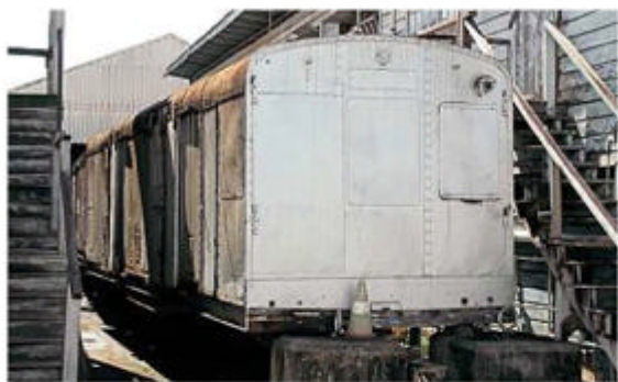
One of two motor freight vans delivered to Bermuda in 1931 – ex-Bermuda Railway petrol railcars 30 or 31 (EE 846 / 847 1931) – in use in September 2014 as stores at the old Georgetown railway workshops, which are still used by the Guyana Government Transport & Harbour Dept. THOMAS KAUTZOR
