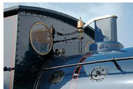
After: The retro-fitted (lower) timber cab roof and dummy Ramsbottom safety valve bonnet. NICK BRODRICK
