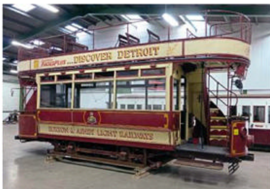
Burton & Ashby Light Railway tram No. 14 displayed in the 'Grain Store' museum building at the Statfold Barn Railway. It will be re-gauged to 2ft and overhauled to run at the SBR during regular open days. Picture: SBR
