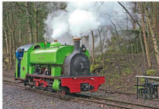
Thomas Green & Company 0-6-2ST Barber steams in the South Tynedale Railway's yard at Alston on February 19 – the first time it has steamed on STR metals. The low cab profile arose from the need to work through a confined tunnel at Harrogate. DAVE HEWITT
