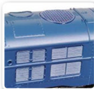
Etched grille & engraved roof fan detailing
