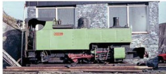
Russell pictured in 1965 when it was on the wharf edge behind the museum at Tallyllyn's station. The leading pony truck had been removed during its time working on Fayles Tramway in Dorset. The locomotive looks very different now, as does the site, with this old museum having been replaced by a magnificent new structure several years ago. DAVID MITCHELL
