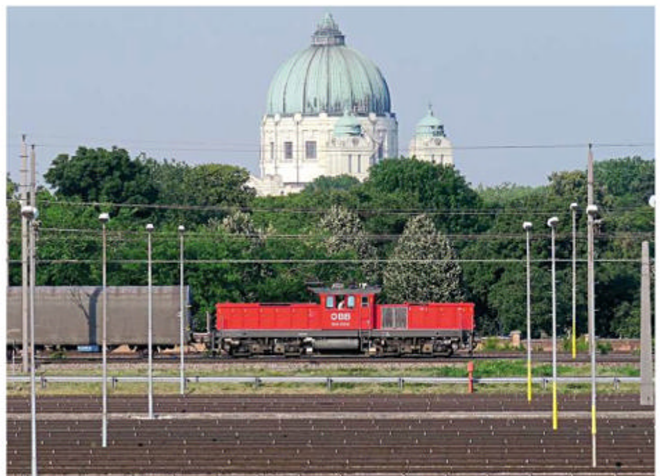
Vienna's Kledering yard uses British-built Dowty retarders. This view of the sorting sidings in June 2013 shows the thousands of Dowty dashpots spread throughout the sidings. An Austrian State Railways Class 1063 Bo-Bo shunter arrives with a transfer freight. Vienna's central cemetery building is in the background.
