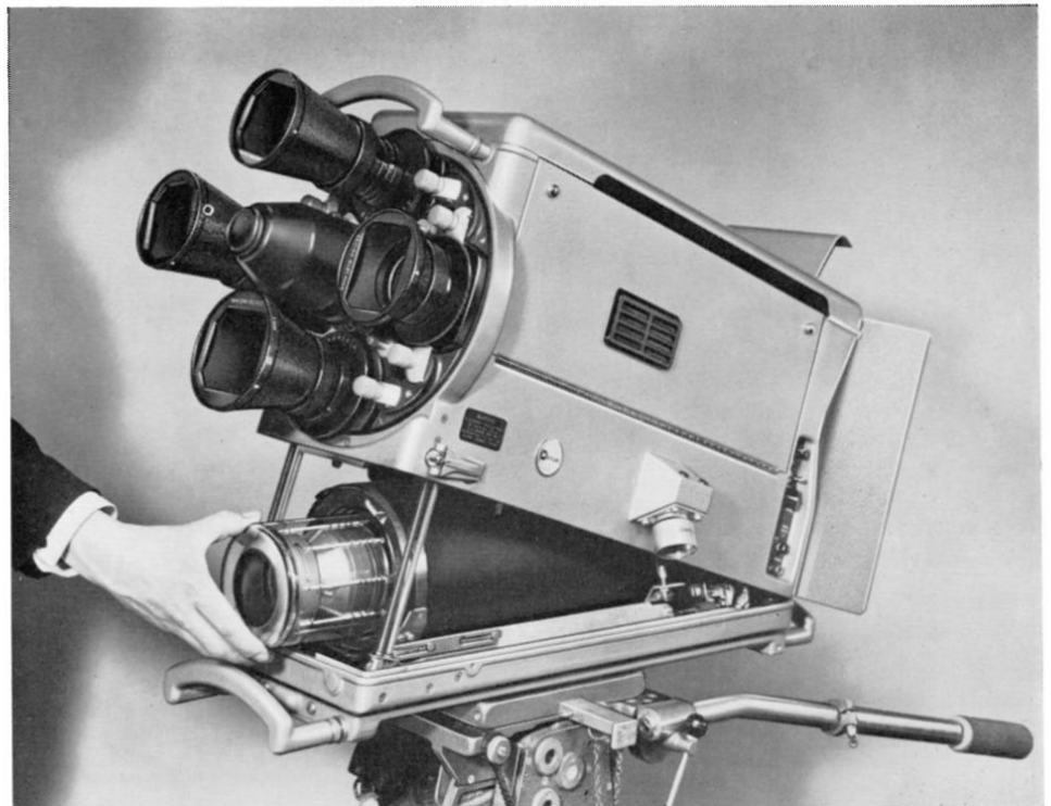
The body of the camera hinged upwards giving excellent access to the image orthicon tube.
