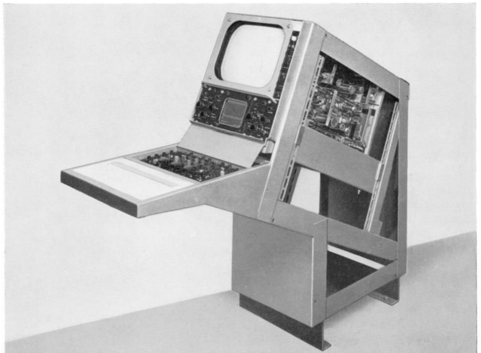
The camera control unit, mounted (horizontal) with a picture and waveform monitor in a standard console.
