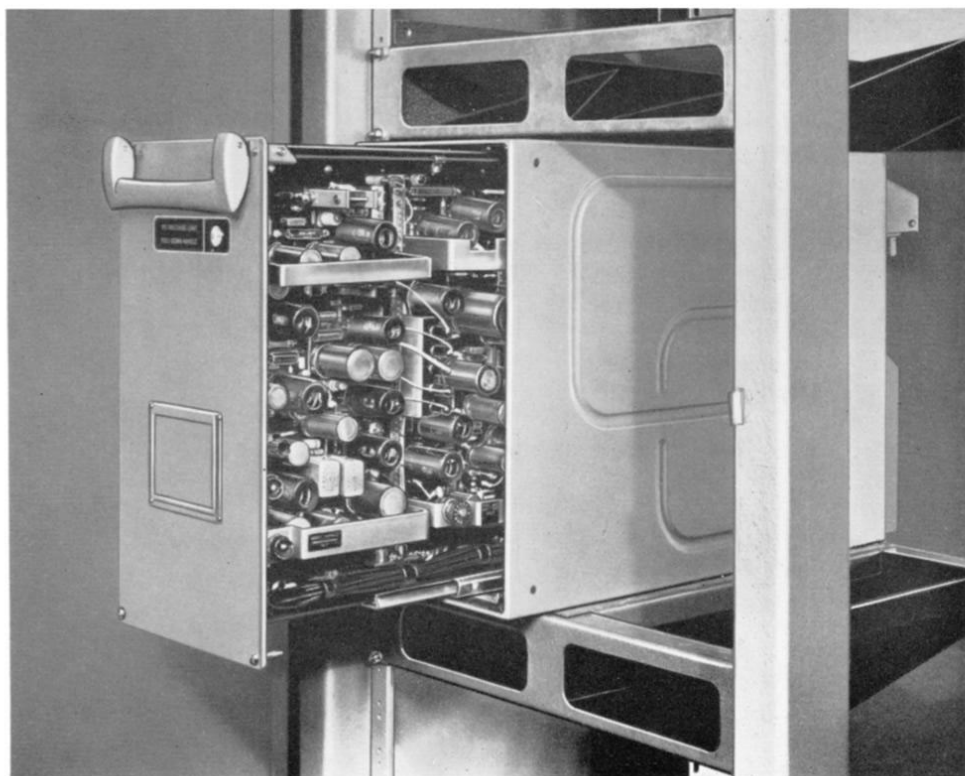
Interior of the camera control unit. Individual boards are readily removable, having plug-in connections. A unique bus-bar system at each side provides mechanical rigidity and a means of feeding HT and heater supplies to the circuits at low impedance.
