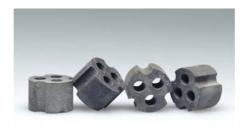
Fig. 7. The Reforming Catalyst
