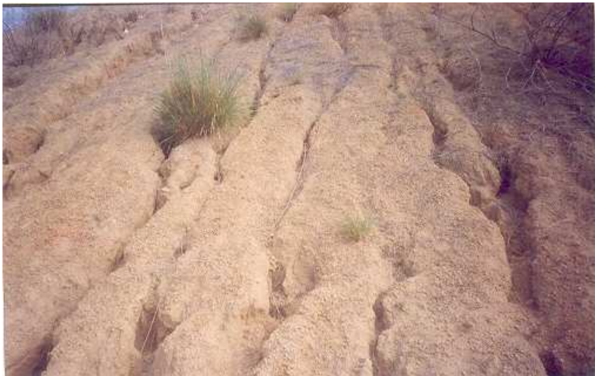
Photo 6: Un-vegetated waste dumps showing development of gullies, Makrana mining area, district Nagaur.
