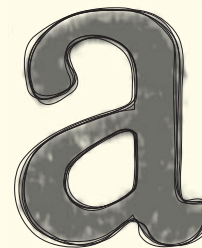
20 Overlaid Bezier curves of five different a's that determine the average shape of the character.
