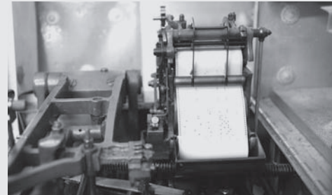
8 Monotype perforated tape on the the keyboard and in the composition caster
