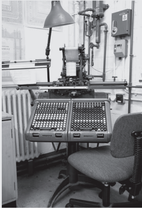
6 Monotype 'D' keyboard, introduced in 1908
