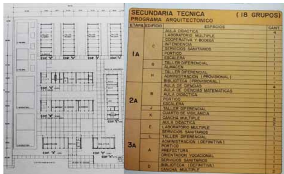
Figure 21. Example of layout of a technical secondary school for 18 groups and typical schedule of accommodation.
