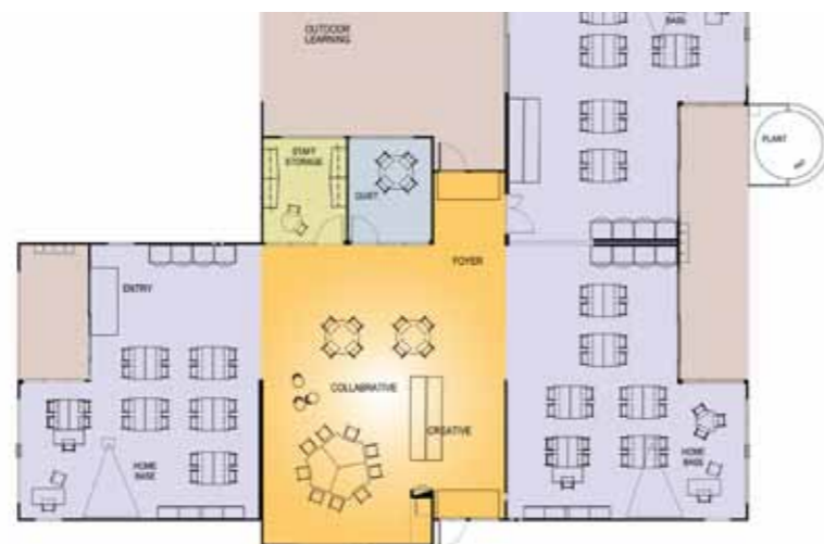
Figure 3. Small school classroom 2. This design includes three classrooms, a project space and administration area. This facility is manufactured offsite, which results in increased quality and minimal disruption to schools.
