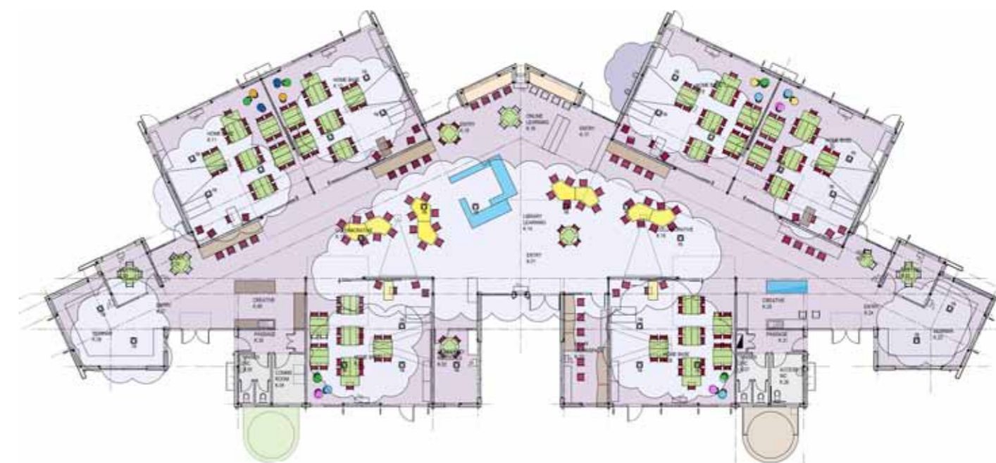
Figure 1. Library and classroom 5. This facility is configured around a centrally located learning resource centre with zones for online learning and small performance and presentation. Six ICT rich home bases link to the central resource centre. Spaces at each end of this facility enable community access, quiet reflection or creative investigation.
