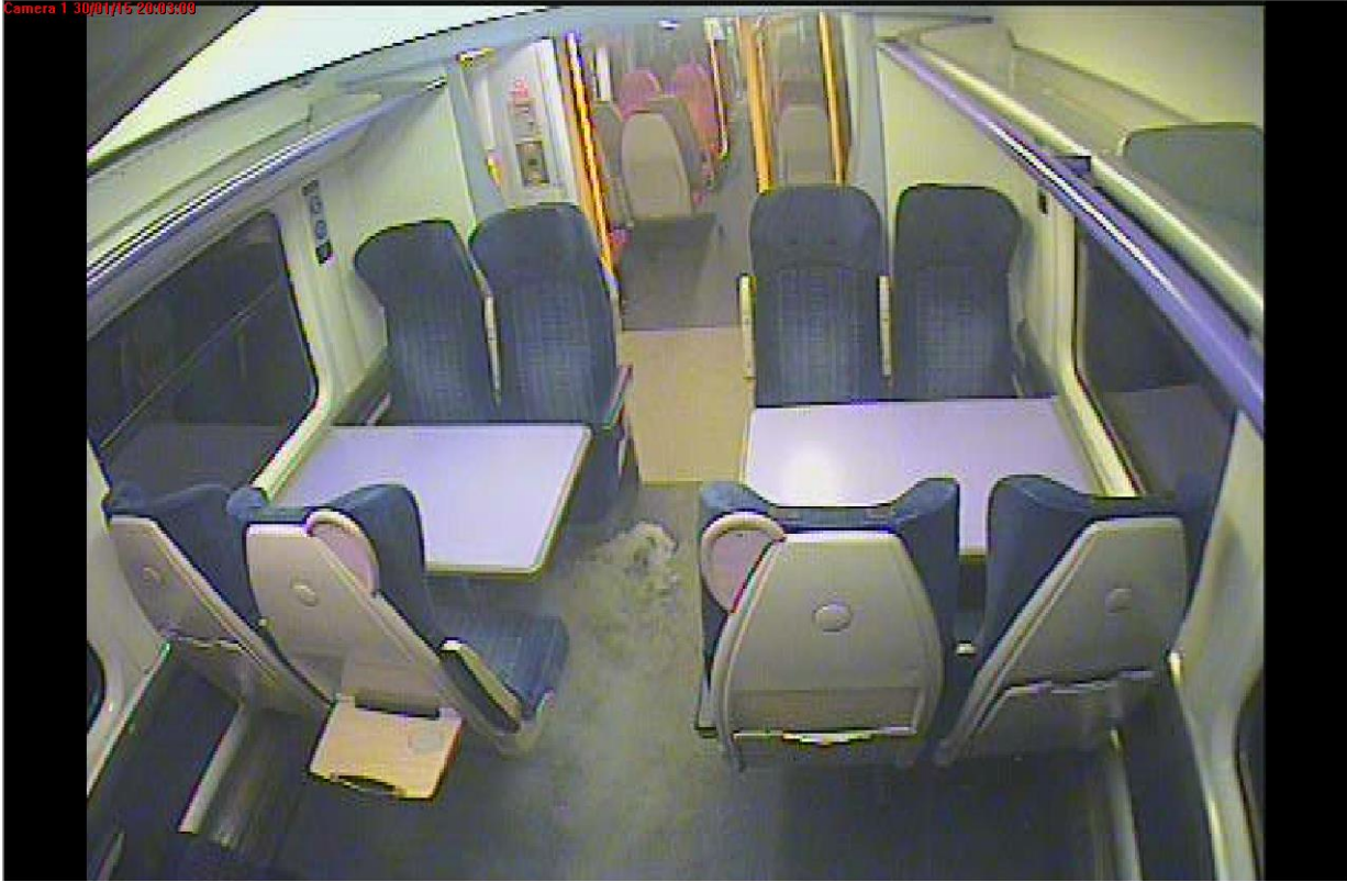
Figure 3: smoke breaks through the floor of carriage 67601
