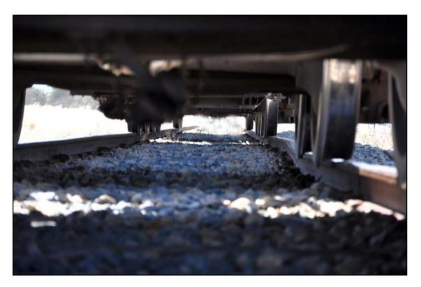
Photograph 2: Buckle visible under the 39th wagon
