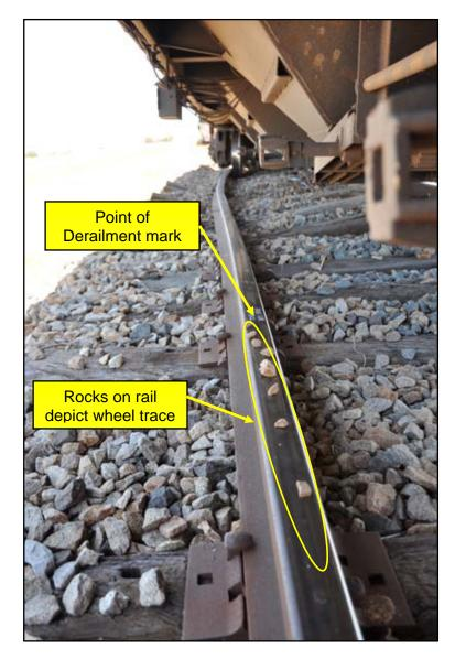
Photograph 1: Point of derailment marks on the Up rail
