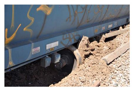
Photograph 3: Wheel from the 36<sup>th</sup> wagon acting as a plough
