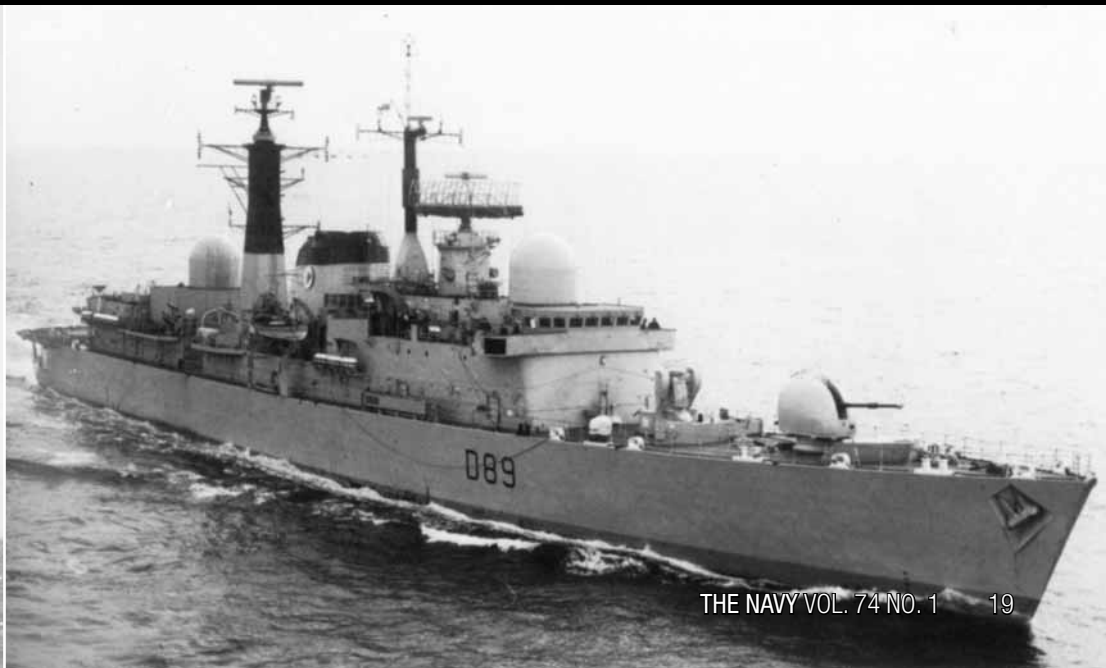
08 HMS EXETER during the Falkland's Conflict. As a Batch II Type 42 destroyer her better combat system allowed her to engage Argentine aircraft at wave top height, something the Argentines knew was a weakness of the Batch I ships deployed. (RN)
