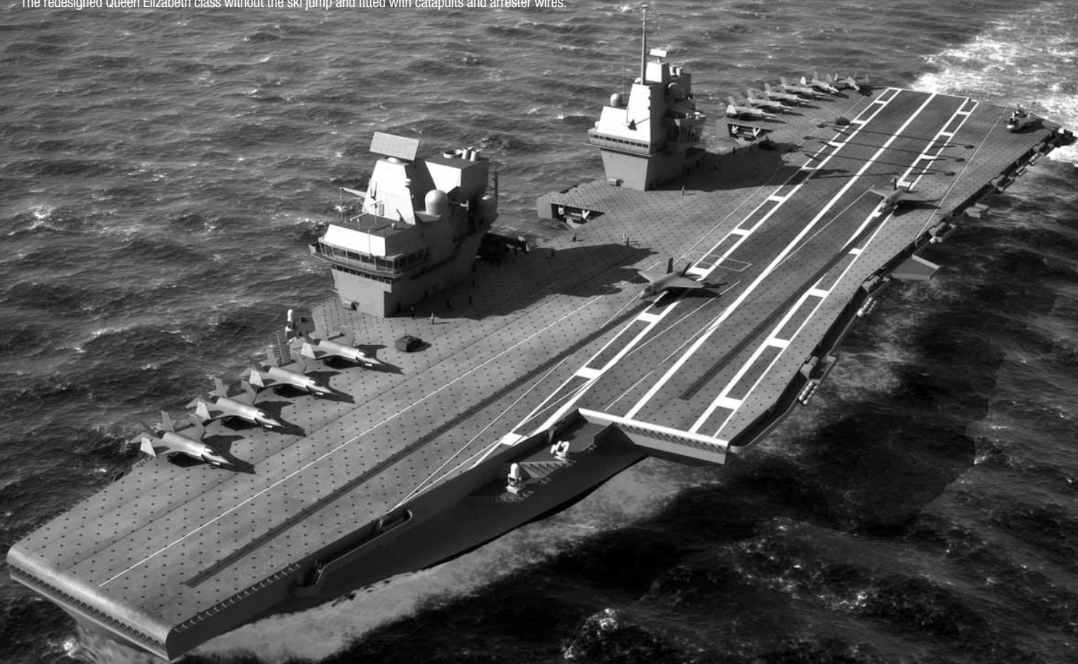
The redesigned Queen Elizabeth class without the ski jump and fitted with catapults and arrestor wires.
