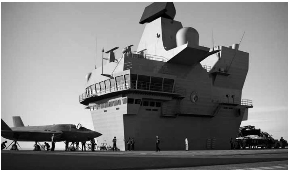
A computer generated image of the forward island superstructure as it will look like from the flight deck.
