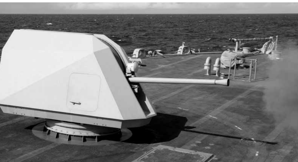
The Bofors 57 mm gun. With a rate of fire of 220rpm the Bofors is one of the best small - medium calibre guns on the market for anti-air and anti-missile roles. With effective lower calibre guns such as these navies could increase the calibre of other gun systems to be more suitable of NGS/anti-surface roles. (USN)
