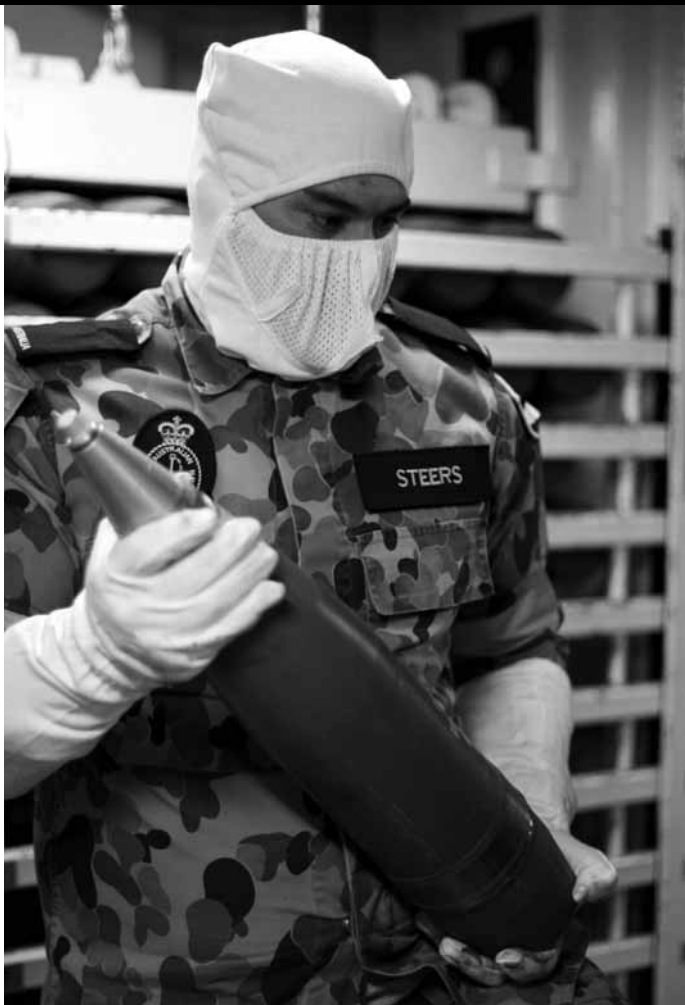
Light enough for one man to pick up, the 5-inch shell as used by the RAN for NGS. Fine for anti-aircraft fire but not so appropriate to support troops in contact for suppression fire. (RAN)
