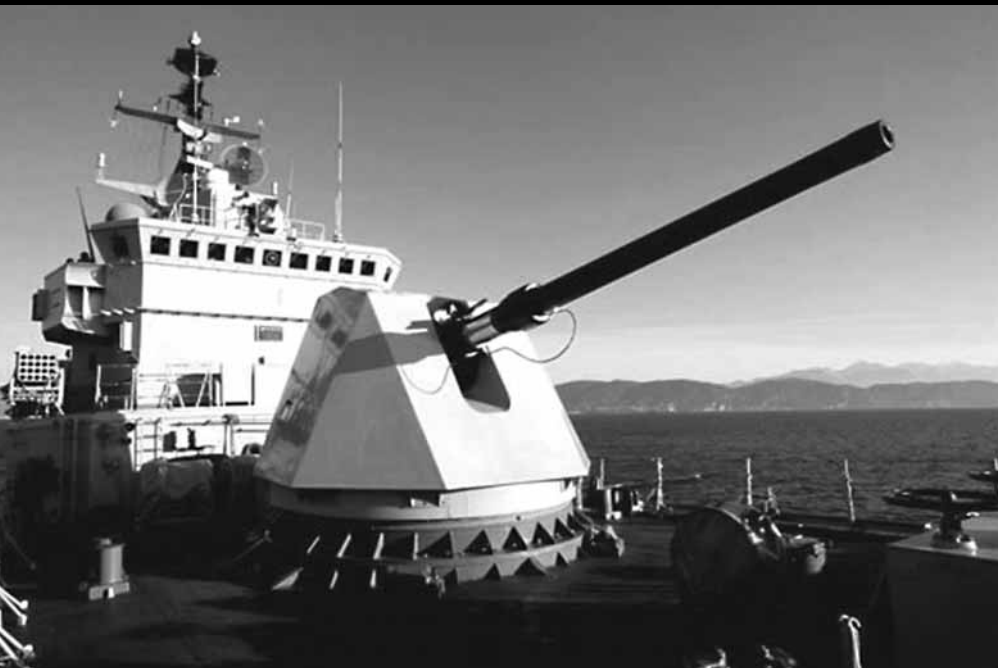
The Italian OTO Melara 127mm/64 lightweight gun. The range and rate of fire of this gun, and its ability to use all existing US 5-inch ammunition, makes it an attractive alternative to the relatively low rate of fire USN Mk-45 series of guns.
