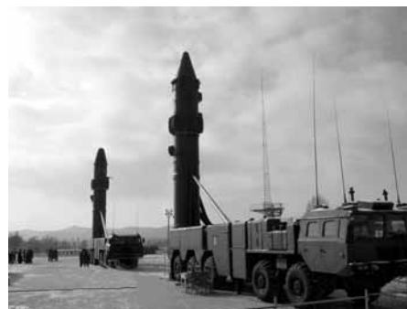
Two Chinese mobile DF-21 Intermediate Range Ballistic Missile launchers. The DF-21 has been modified by the Chinese with a radar seeker and control fins to attack ships far out to sea from China's mainland. This is the first guided anti-ship ballistic missile and presents the problem of high angle (coming from almost above) and high speed. Only BMD fitted ships will be able to defend against it.
