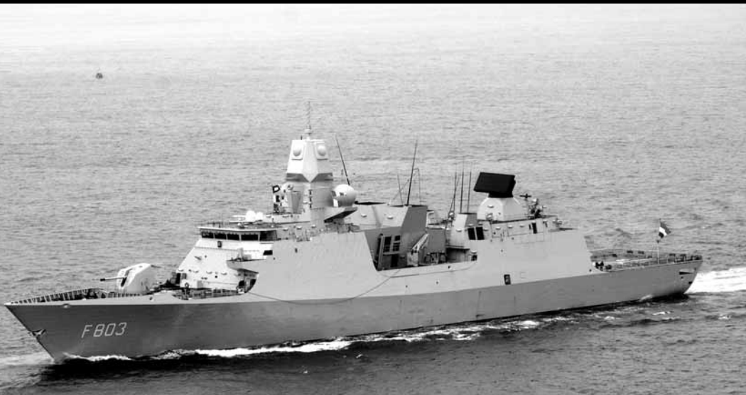
06 The Dutch Frigate TROMP in Sydney Harbour. The class's SMART-L long range surveillance radars will be upgraded in order to detect and track ballistic missiles. (Chris Sattler)
