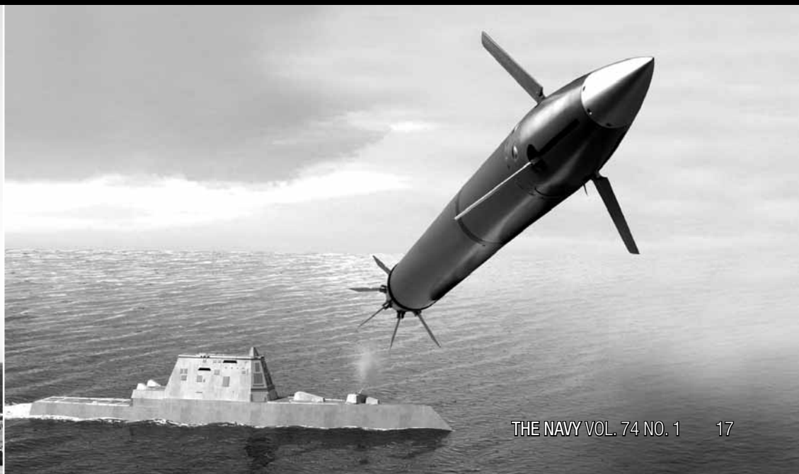
05 A computer generated image of the USN's 155mm Long Range Land Attack Projectile (LRLAP) fired from the 155 mm (6.1 inch) AGS on a Zumwalt-class (DDG-1000) destroyer.
