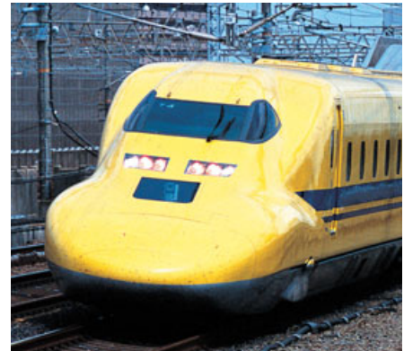
▲High-Speed Multipurpose Inspection Train (Doctor Yellow)
