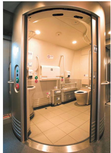
▲Multifunction Toilet Space (with ostomate-accessible facility)
