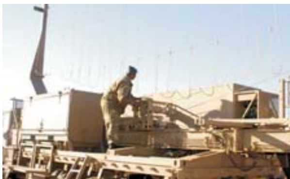
The recovery vehicle with its net or series of ropes provides the runway for automatic landing.
