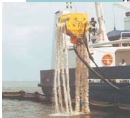
When the sea mop is dragged through the oil, it can remove up to 15 tons of oil per hour.
