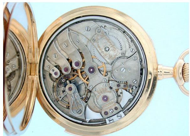
This picture shows the two gong rods curling round the outside, clamped between the two hammers.
