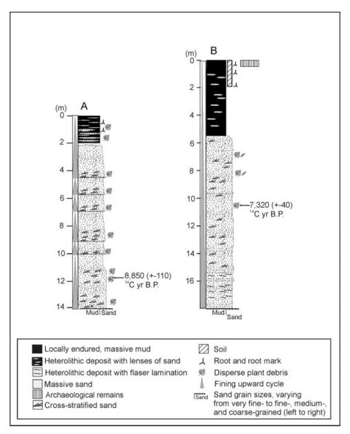
**Figure 4.** (a, b) Lithostratigraphic profiles representative of two paleochannels in Marajó Island. Note the prevalence of sand deposits at the base, which grade upward into muds, forming fining-upward cycles, the recorded radiocarbon ages suggesting channel fill during the early Holocene, and the human artifacts at the top of profile 4b.
