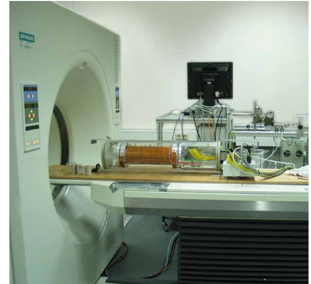
Spiral CT technology in combination with core flooding, Shell Technology Centre Rijswijk, the Netherlands
