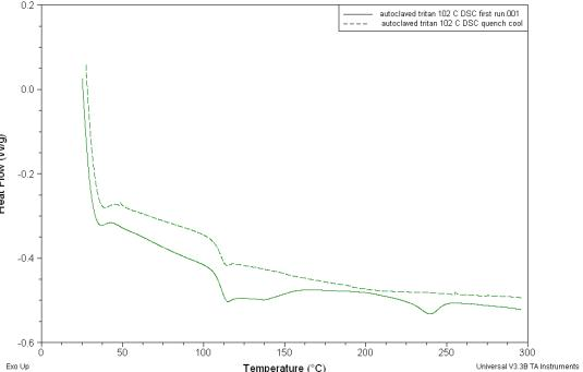
Heat Flow vs. Temperature Graphs for Tritan <sup>™</sup> Copolyester Bottles Autoclaved at 102°C
