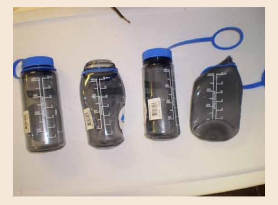
• 1) New Tritan <sup>™</sup> copolyester bottle. 2) After 1 hour ramping from 25 to 125 C. 3) 2 hours in autoclave at 102 C. 4) 2 hours in autoclave at 121 C.
