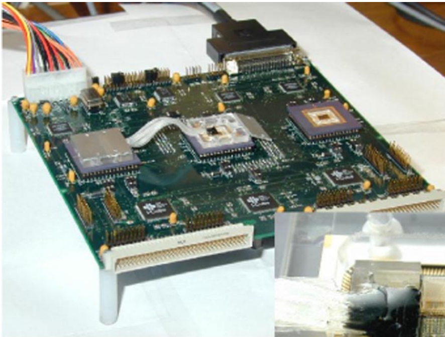
Figure 15. The opto-electronic FPGA demonstrator. Inset: partially packaged Opto-electronic FPGA.
