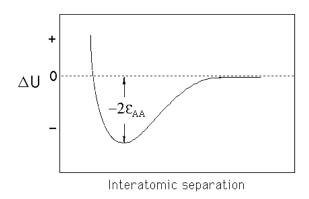
Fig. 3: Curve showing schematically the change in energy as a function of the distance between a pair of A atoms.  $-2\epsilon_{AA}$  is the binding energy for the pair of atoms. There is a strong repulsion at close-range.
