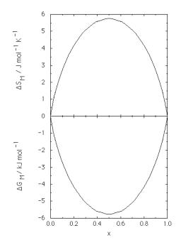
Fig. 2: The entropy of mixing and the free energy of mixing as a function of concentration in an ideal binary solution where the atoms are distributed at random. The free energy is for a temperature of 1000 K.
