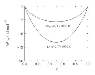
Fig. 4: The free energy of mixing as a function of concentration in a binary solution where there is a preference for unlike atoms to be near neighbours. The free energy curve for the ideal solution ( $\Delta H_M = 0$ ) is included for comparison.
