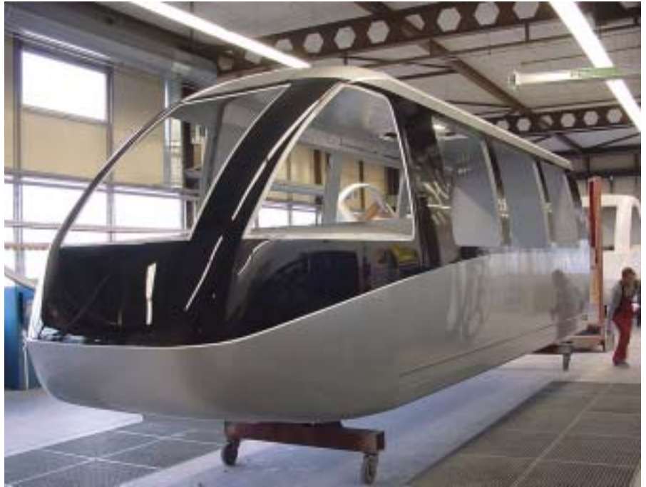
The SDI-designed People Mover train bodies were hand-crafted from aviation grade structural aluminum.
