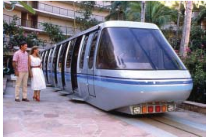
SDI built the Waikoloa Hilton (then, Hyatt) Hawaii People Mover in 1987 using first generation UniTrak technology.
