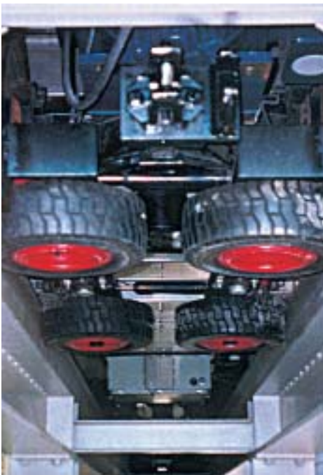
Each People Mover train is powered by four on-board propulsion bogies that consist of a variable-frequency AC Drive, Rockwell Axle Assembly, transmission, drive wheels and guide wheel assembly.
