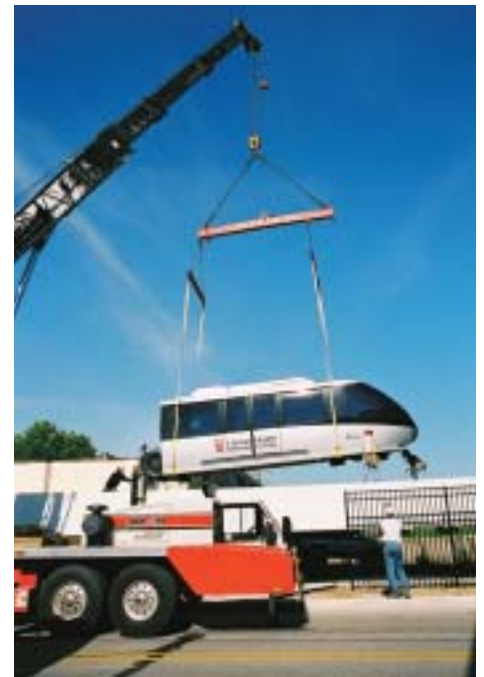
The Clarian People Mover's four 'nose' cars are 28-feet long — six feet longer than the two center cars.
