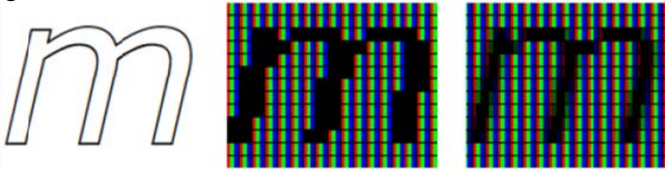
FIGURE: (a) letter 'm' in italic (left) (b) whole-pixel rendered 'm' with jagged edges (middle) (c) subpixel rendered 'm' with smooth edges (right)
