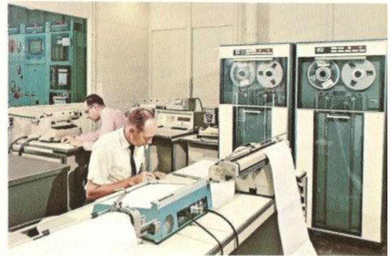
Information which is needed immediately by the reactor operator is displayed on the main control panel (above). Auxiliary instruments not requiring constant surveillance are located in other areas. Below, a digital computer and data handling equipment are utilized to provide current information on important variables within the reactor system.
