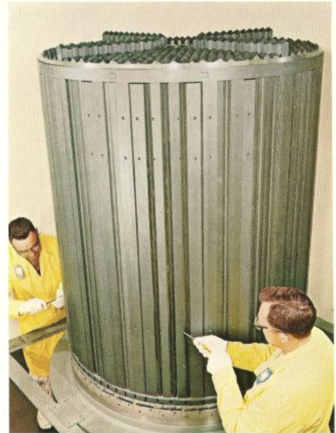
The reactor core, shown while being assembled, contains 69 cubic feet of graphite. The 1,140 fuel channels contain about 20 cubic feet of molten salt fuel when the reactor is in operation.
